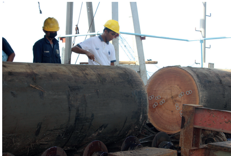
Hammering metal plates into meranti logs to reduce end-splitting at a log yard in Probolinggo, Indonesia prior to peeling for plywood. ITTO is undertaking Environmental Product Declarations for meranti plywood and other tropical timber products. Photo: MY Massijaya
