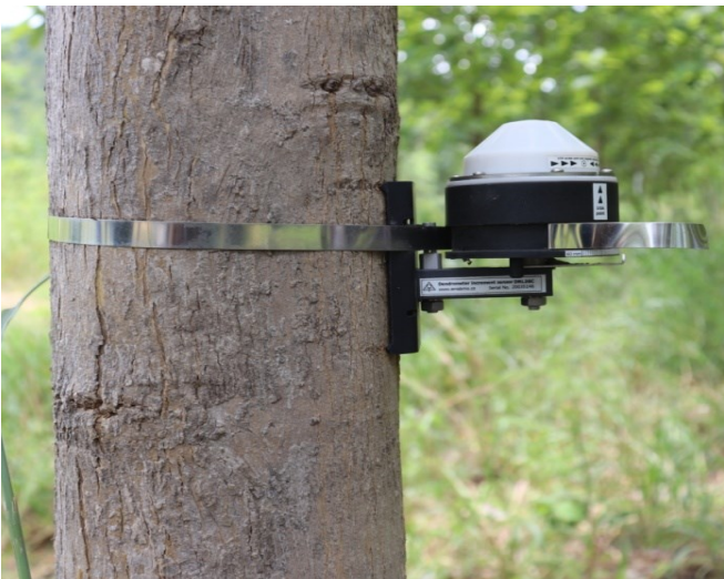
Change in dimension of tree trunk monitored through dendrometer
