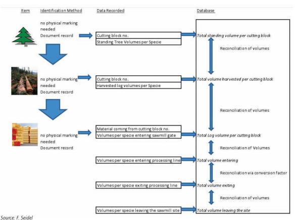
Figure 4: Illustrated concept of a mass balance system
