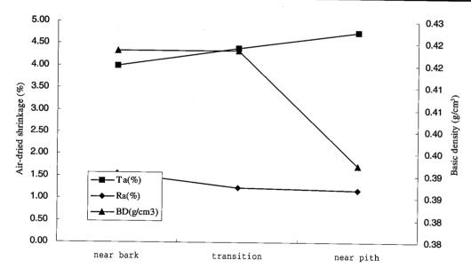
Fig.1.2-2 *A.magnium*: relationship between air-dried shrinkage (Ta&Ra), basic density (BD) and different radial positions
