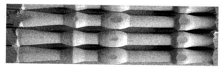
Fig.3.2-14 Turning samples after sanding
