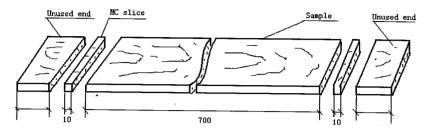
Fig.5.1-1 Drying sample making of E. citriodora
