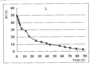
Fig.4.2-3 MC curve in 100°C-test of E. exserta
