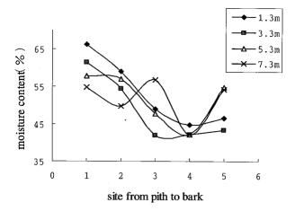
Fig.1.2-1 Variation in moisture content of E. citriodora green wood at different tree heights and different radial sites
