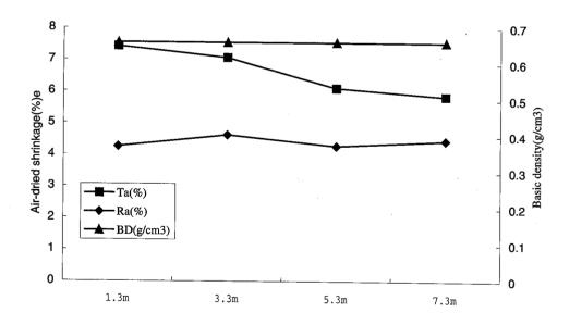
$Fig. 1.2-2 \textit{E.teretiocornis} : \ relationship \ between \ air-dried \ shrinkage \ (Ta\&Ra), \ basic \ density \ (BD) \ and \\ tree \ heights$
