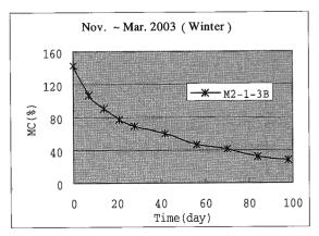
Fig.3.1-3 The air-drying MC curve of Acacia magium
