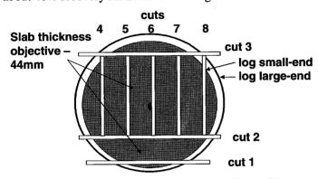
Fig. 4.5-1 Sawing strategy of log in 25 cm diameter
