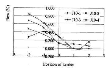
Fig. 3.2-2 The bow deformation of E. grandis in cant sawing
