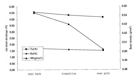
Fig.1.2-3 *A.auriculiformis*: relations between air-dried shrinkage, basic density and different radial positions
