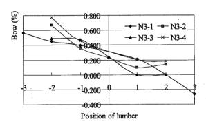
Fig. 4.2-2. The bow deformation of E. citriodora in cant sawing
