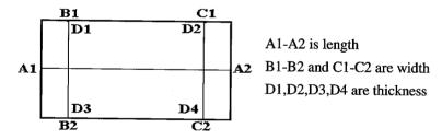
Fig.3.2-1 The dimension measure in 100 ℃-test of Acacia magium
