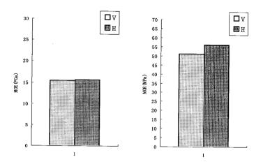
Fig.5.1-8 Comparison between V-type and H-type finger-joints on MOE and MOR
