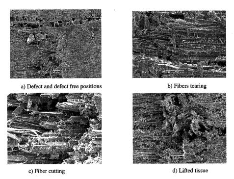
Fig.3.2-2 SEM observation of planning defects of E. citriodora
