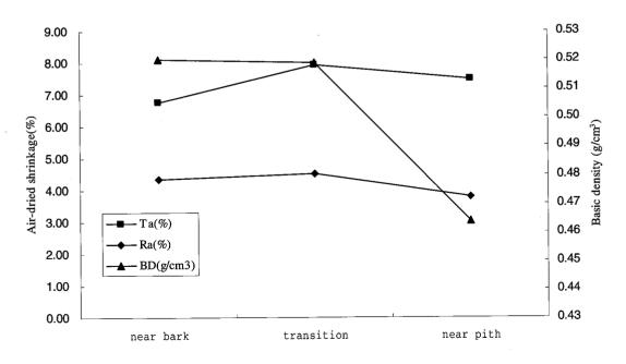
Fig.1.2-3E.urophylla × grandis: relationship between air-dried shrinkage (Ta&Ra), basic density (BD) and different radial positions
