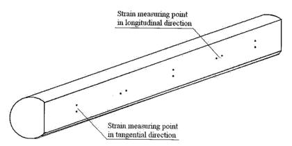
Fig. 3.1-2 Distribution of measuring point for strain change in lumber sawing
