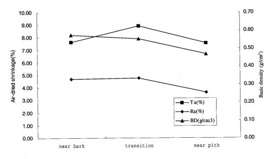
Fig.1.2-3 *E.urophylla*: relationship between air-dried shrinkage (Ta&Ra), basic density (BD) and different radial positions
