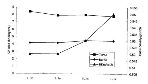
Fig.1.2-2 *E.urophylla*: relationship between air-dried shrinkage (Ta&Ra), basic density (BD) and tree heights
