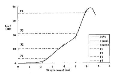
Fig.6.1-5. Load-displacement curve
