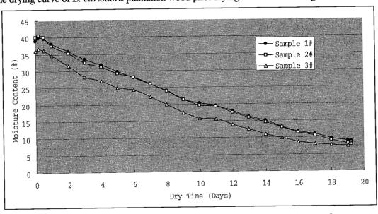
Fig. 5.4-1 The drying curve of E. citriodora plantation wood
