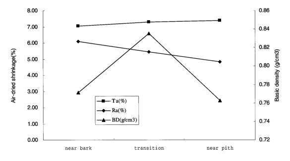
Fig.1.2-3 E. citriodora: relationship between air-dried shrinkage (Ta&Ra), basic density (BD) and different radial positions
