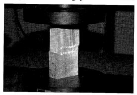
Fig.6.1-1. The method of measuring end-pressure
