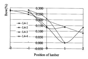
Fig. 3.2-1 The bow deformation of E. exserta in live sawing
