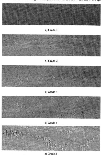
Fig.3.2-1 Grades 1 to 5 torn grain samples of E. citriodora
