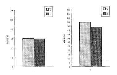
Fig.5.1-7 Comparison between V-type and H-type finger-joints on MOE and MOR
