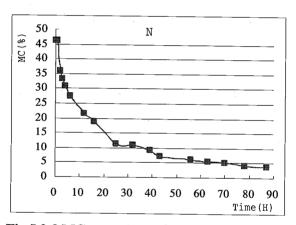
Fig.5.2-3 MC curve in 100 °C-test of E. citriodora
