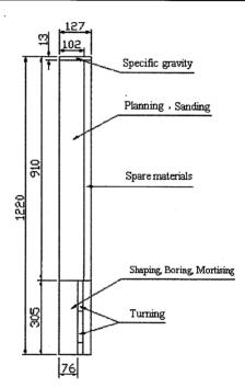
Fig.3-1 Diagram for sawing lumber into smaller samples for individual tests
