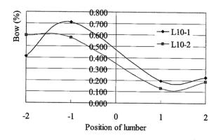
Fig. 3.2-2 The bow deformation of *E. exserta* in cant sawing
