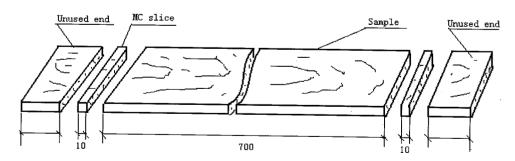
Fig.4.1-1 Drying sample making of E. grandis
