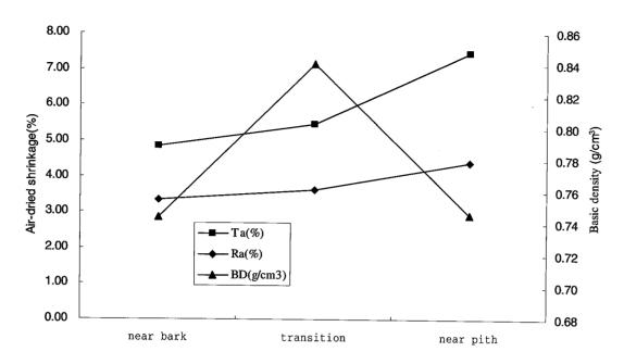
Fig.1.2-1 *E. exserta*: relationship between air-dried shrinkage (Ta&Ra), basic density (BD) and different radial positions
