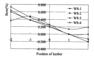
Fig. 4.2-2 The bow deformation of E. urophylla× grandis in cant sawing
