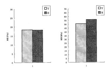
Fig. 6.1-7 Comparison between V-type and H-type finger-joints on MOE and MOR
