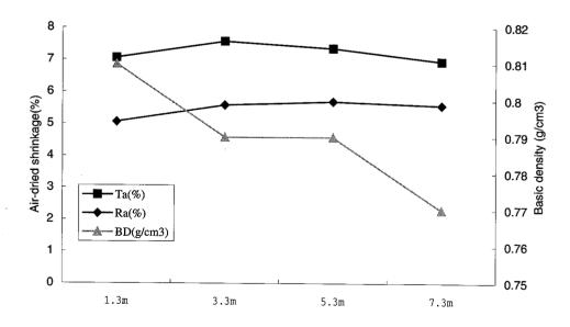
Fig.1.2-2 Relationship between air-dried shrinkage, basic density and tree heights
