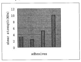
Fig.5.2-1 Shear strength comparisons of 4 adhesives
