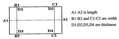
Fig.4.2-1 The dimension measure in 100 ℃-test of E. grandis
