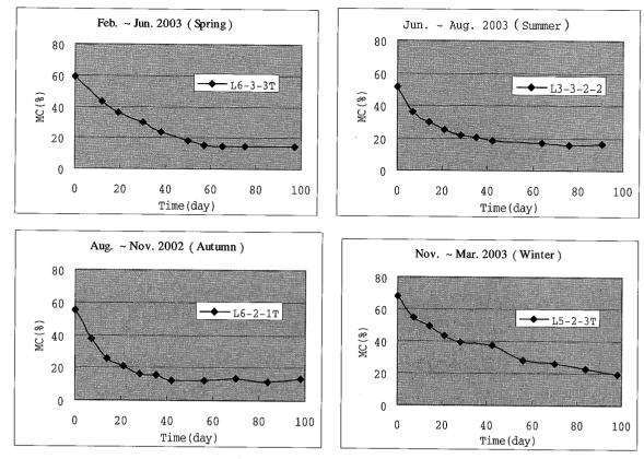
Fig.5.1-3 The air-drying MC curve of E. exserta
