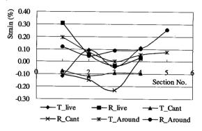
Fig. 4.1-3 Strain distribution of E. citriodora in tangential and radial direction
