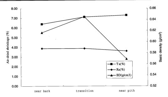
Fig.3-2-16 *E.pellita*: relationship between air-dried shrinkage (Ta&Ra), basic density (BD) and different radial positions
