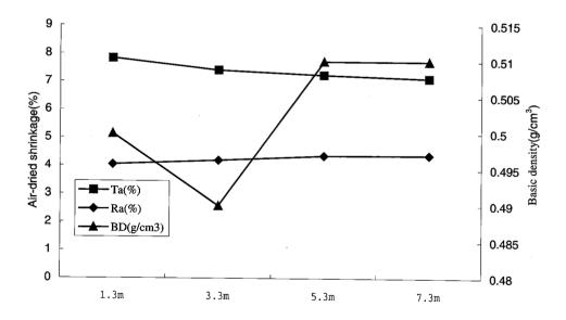
Fig.1.2-2*E.urophylla*×*grandis*: relationship between air-dried shrinkage (Ta&Ra), basic density (BD) and tree heights
