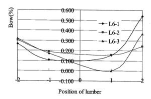
Fig. 3.2-3 The bow deformation of E. exserta in around sawing
