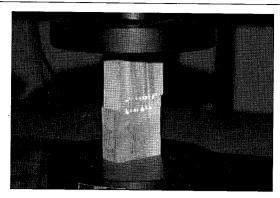
Fig.5.1-1. The method of measuring end-pressure
