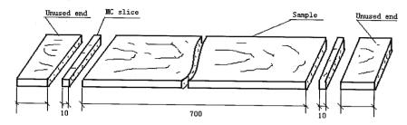
Fig.3.1-1 Drying sample making of Acacia magium
