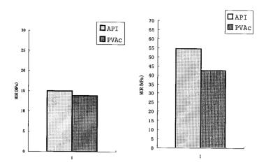
Fig.5.1-8 Comparison between API and PVAc finger-joint on MOE
