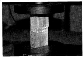
Fig.5.1-1. The method of measuring end-pressure
