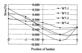
Fig. 4.2-1 The bow deformation of E. urophylla× grandis in live sawing
