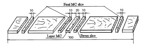
Fig.4.1-2 MC slices making of E. exserta
