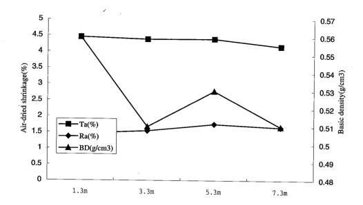
Fig.1.2-2 A.auriculiformis: relationship between air-dried shrinkage, basic density and tree heights
