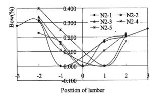
Fig. 4.2-3. The bow deformation of E. citriodora in around sawing
