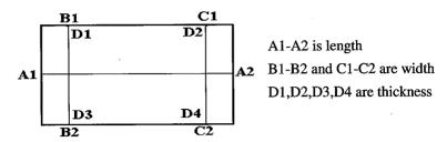
Fig.4.2-1 The dimension measure in  $100\,\mathrm{^{\circ}C}$ -test of E. exserta
