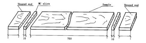
Fig.4.1-1 Drying sample making of E. exserta
