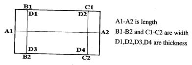
Fig.5.2-1 The dimension measure in  $100\,^{\circ}$ C-test of *E. citriodora*
