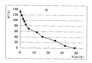
Fig.3.2-3 MC curve in 100 °C-test of Acacia magium
