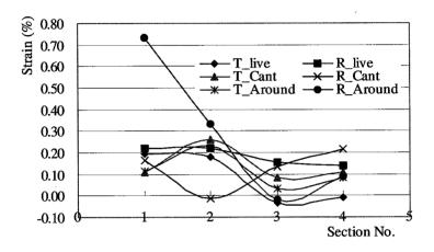
Fig. 3.1-3 Strain distribution of *E. grandis* in tangential and radial direction
