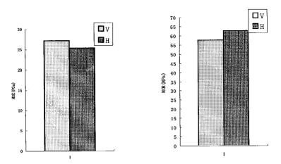
Fig.6.1-8. Comparison between V-type and H-type finger-joints on MOE and MOR
