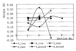
Fig. 3.1-3 Strain distribution of E. exserta in tangential and radial direction
