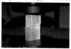
Fig.6.1-1 The method of measuring end-pressure
