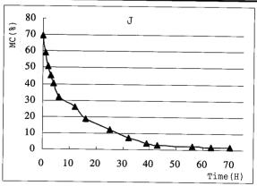
Fig.4.2-3 MC curve in 100 °C-test of E. grandis
