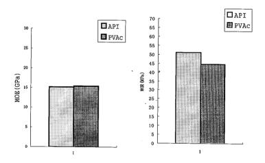
Fig.5.1-9 Comparison between API and PVAc finger-joint on MOE
