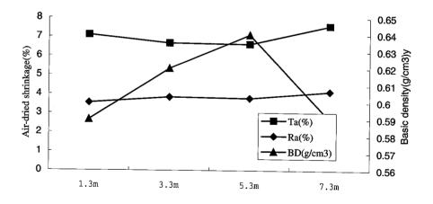
Fig.1.2-2 *E.pellita*: relationship between air-dried shrinkage (Ta&Ra), basic density (BD) and tree heights
