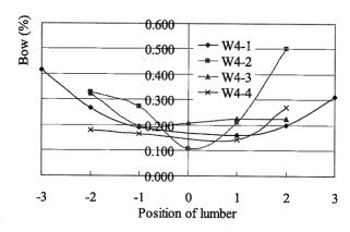
Fig. 4.2-3 The bow deformation of *E. urophylla× grandis* in around sawing
