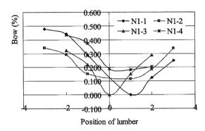
Fig. 4.2-1. The bow deformation of E. citriodora in live sawing
