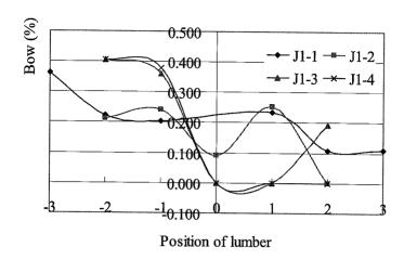
Fig.3.2-1 The bow deformation of E. grandis in live sawing
