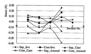
Fig. 4.1-4 Strain distribution of E. citriodora in longitudinal direction
