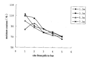
Fig.1.2-1 Moisture content of green wood for E. cloeziane at different heights and sites
