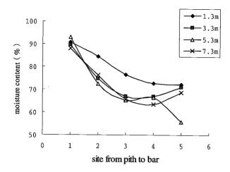
Fig.1.2-1 Moisture content of green wood for E. pellita at different heights and sites
