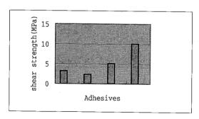
Fig.6.2-1 Shear strength comparison of 4 adhesives
