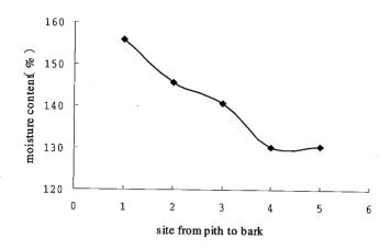
Fig.1.2-1 Moisture content of green wood for A. magnium at different sites
