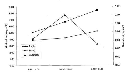
Fig.1.2-3 *E.tereticornis*: relationship between air-dried shrinkage (Ta&Ra), basic density (BD) and different radial positions
