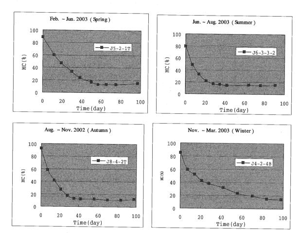
Fig.4.1-3 The air-drying MC curve of E. grandis
