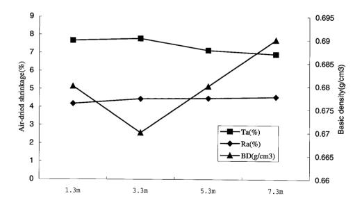
Fig.1.2-2 *E.cloeziane*: relations between air-dried shrinkage (Ta&Ra), basic density (BD) and tree heights
