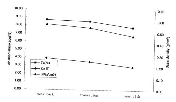
Fig.1.2-1 *E. grandis*: relationship between air-dried shrinkage (Ta&Ra), basic density (BD) and different radial positions
