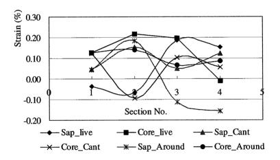
Fig. 3.1-4 Strain distribution of E. grandis in longitudinal direction
