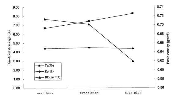
Fig.1.2-3 *E.cloeziane*: relationship between air-dried shrinkage (Ta&Ra), basic density (BD) and different radial positions
