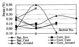
Fig. 3.1-4 Strain distribution of E. exserta in longitudinal direction
