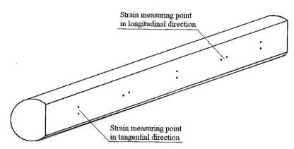
Fig. 4.1-2 Distribution of measuring point for strain change in lumber sawing
