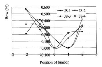
Fig. 3.2-3 The bow deformation of E. grandis in around sawing
