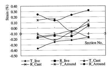
Fig. 4.1-3 Strain distribution of E. urophylla×grandis in Tangential and Radial direction
