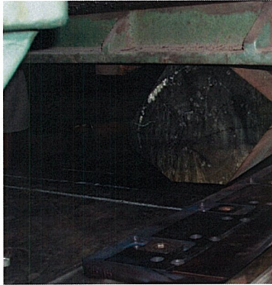
Picture 5 Optimizing sliced veneer recovery by slicing from a 3rd set of parallel sides
