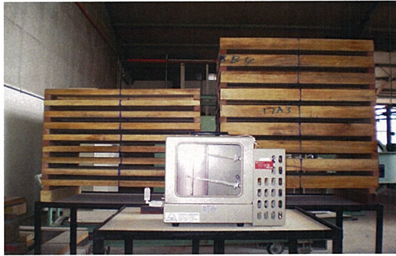
Figure 3 Both the 27- and 54-mm thick Shorea macrophylla test boards sitting on 30" high metal platform for the air-dry test with air conditions recorded by a thermohygrometer
