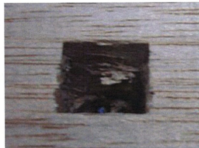
Figure 15 Tearing from mortising test
