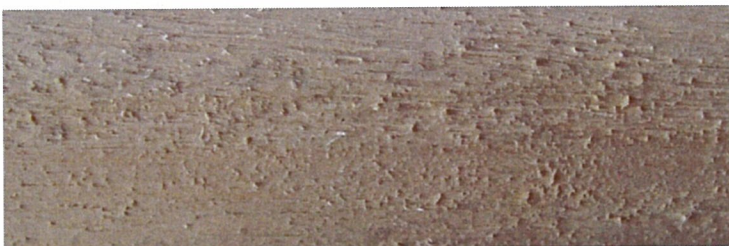
Figure 16 Fuzzy grain as shaping defect
