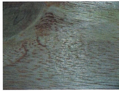
Figure 10 Torn grain from planing test
