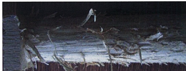
Figure 19 Turning defect of torn grain
