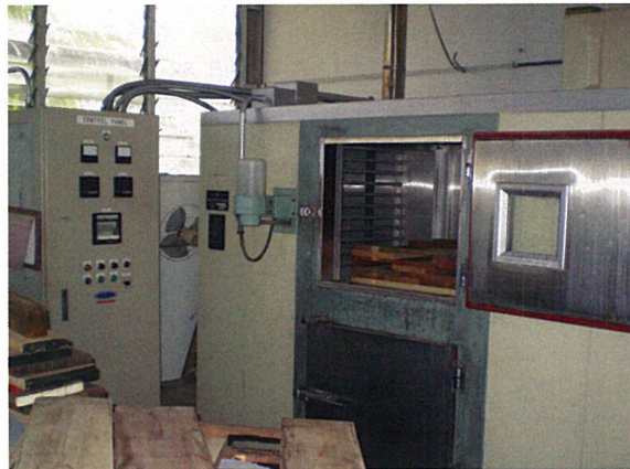
Figure 1 The experimental dryer used to conduct the schedule test
