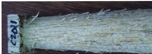
Figure 18 Turning defect of fuzzy grain
