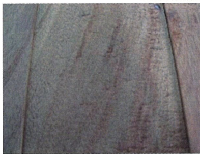
Figure 9 Fuzzy grain from planing test
