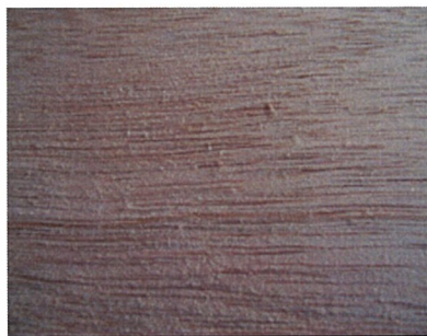
Figure 11 "Fuzzing" defect of sanding test
