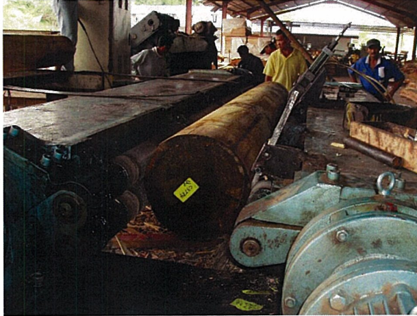
Figure 1 Peeling on an industrial rotary spindle-less veneer lathe
