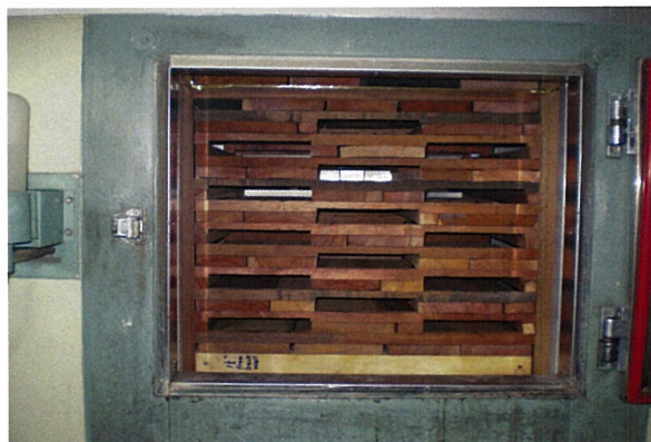
Figure 2 The experimental dryer with dummy stack of 15 slot-in pockets for inserting samples under test in the schedule test
