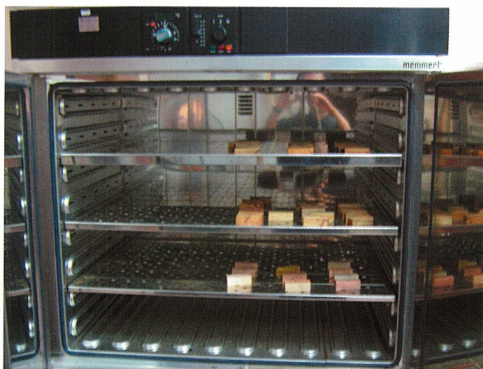
Figure 23 Determination of SG and density by the oven-dry method
