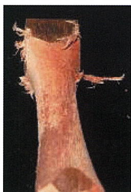
Figure 19 Turning defect of fuzzy grain
