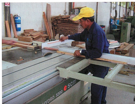
Figure 3 Each stick cut into test specimen sizes according to BS 373
