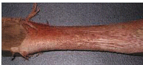
Figure 20 Turning defect of torn grain
