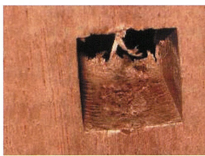
Figure 16 Tearing from mortising test
