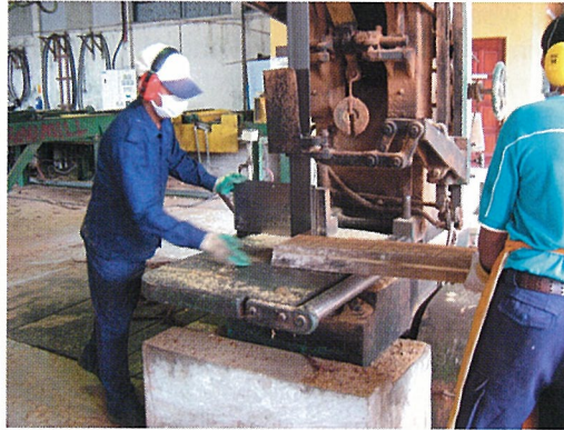
Figure 4 Band-saw used to cut each flitch into sticks
