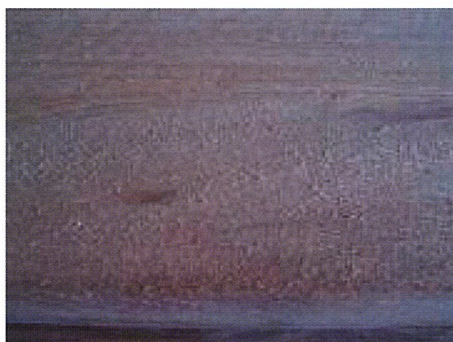
Figure 12 “Fuzzy” defect of sanding test
