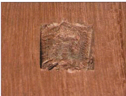
Figure 15 Crushing from mortising test
