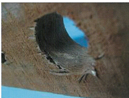
Figure 13 Tear-outs from boring test
