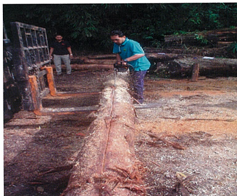
Figure 4 Cutting a groove throughout the length of the log using a chain-saw
