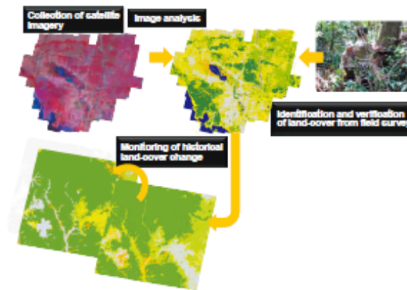
Figure I03-1 Measurement of forest cover changes and emissions and removals per unit of land area
