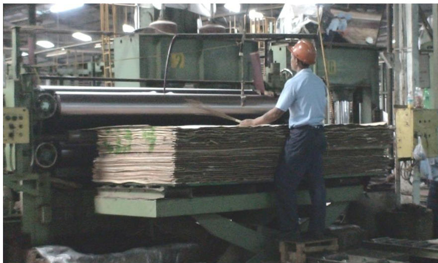
Figure 7. Glue spreading process.
