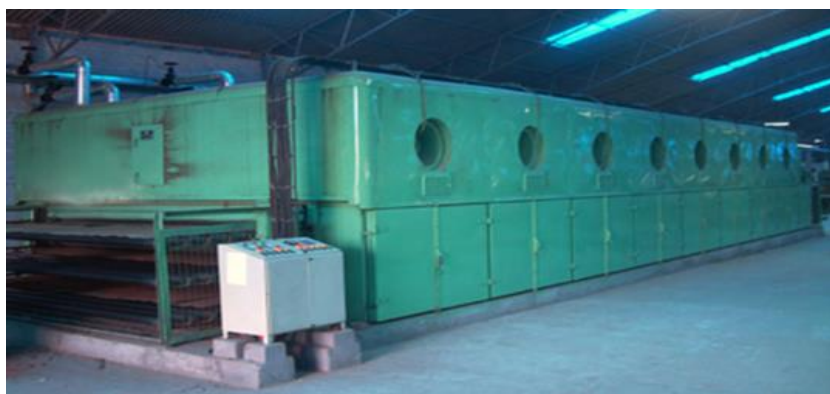
Figure 7. Continuous veneer drying.
