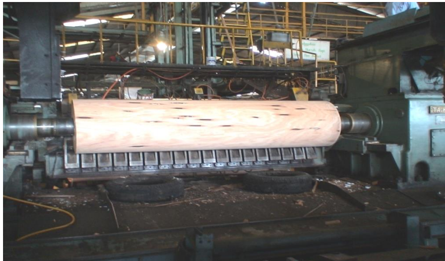
Figure 6. Peeling process of meranti log.
