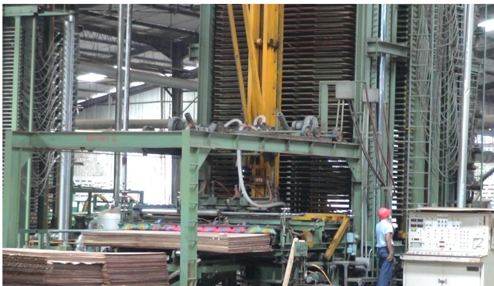
Figure 8. Hot pressing of plywood
