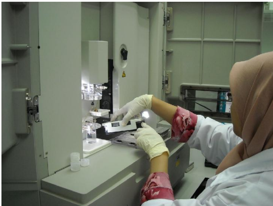
Amplified PCR products are load in ABI 3130x1 Genetic Analyzer System for fragment analysis
