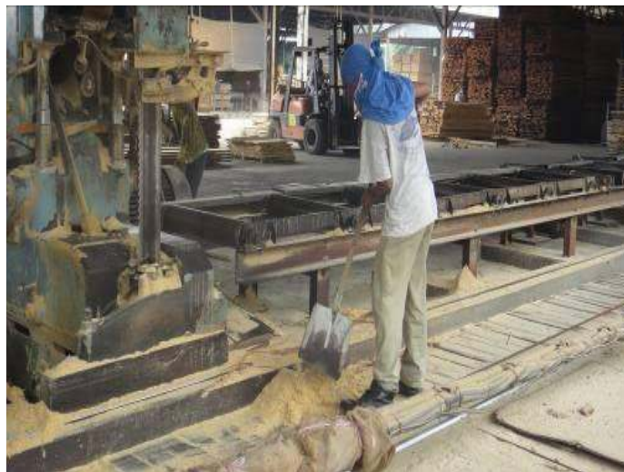
Figure 15: Saw dust collection.
