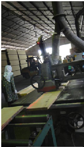
Figure 4: Laser guided sawn timber processing measurement.
