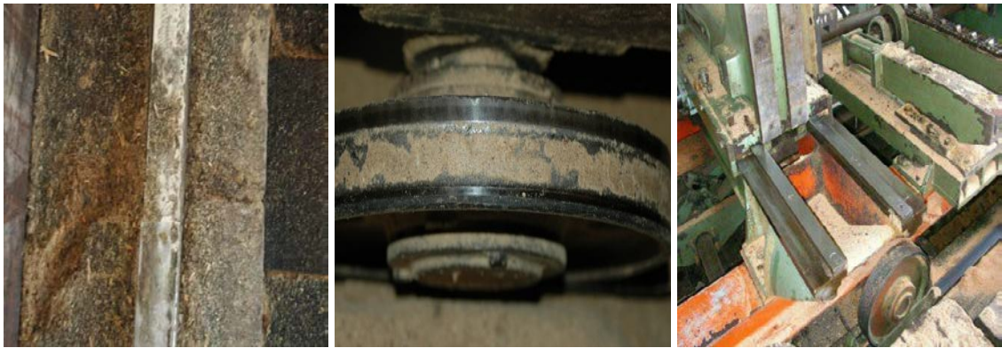
(7) (8) (9) Photos 7-9 (by Kim): damaged rail (7), wheel without scraper (8), unattended log carriage (9)
