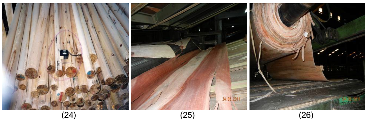
Photos 24-26 (by Kim): use of old-fashioned rotary machine (24), torn veneers due to dull or damaged knives (25), or unmatched speeds of peeling and rolling (26)
