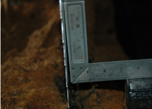
Figure 7: Bandsaw not perpendicular to stopper and fork (Photo by ISWA)
