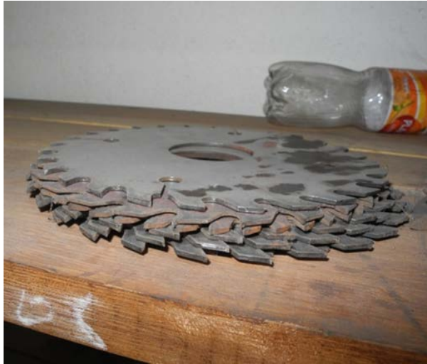
Figure 9: Improper placing of circular saws (Photo by Sukiman)
