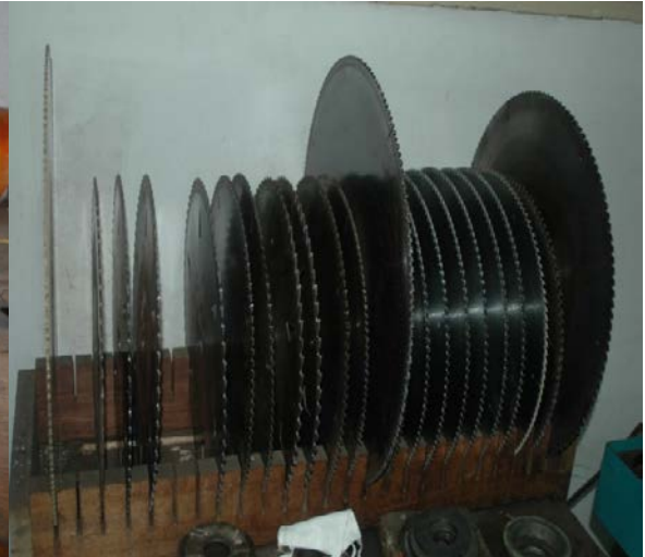
Figure 10: Proper storage of circular saws (Photo by Sukiman)
