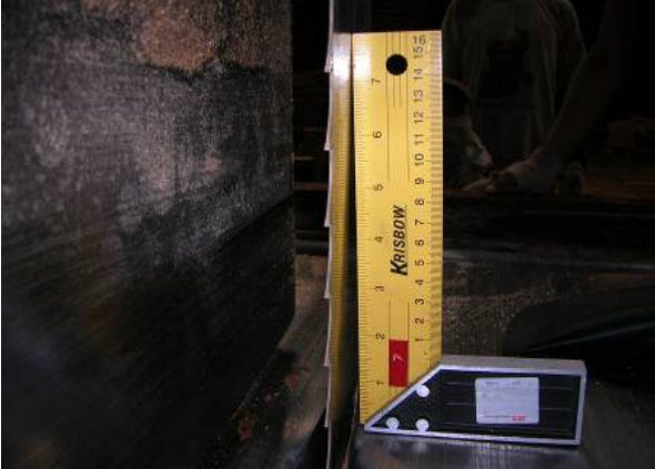
Figure 8: Bandsaw not perpendicular to sawing table (Photo by ISWA)
