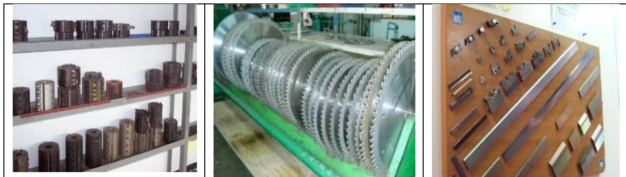
The proper way of storing cutter blocks ; circular saws; and molder knives
