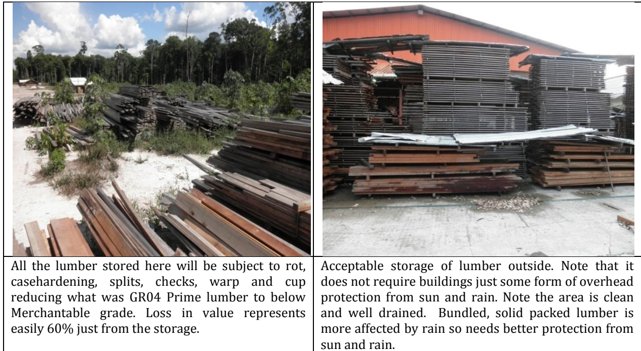
Figure 24: Proper and improper storage of lumber
