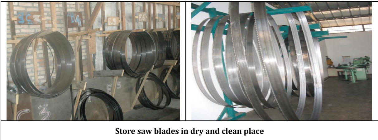
Figure 21: Storage of blades
