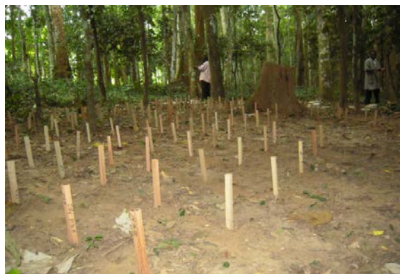
Figure 7.2: Samples planted in the graveyard test site with termite mount
