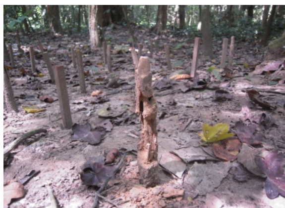
Figure 7.6: Test samples infested with termites
