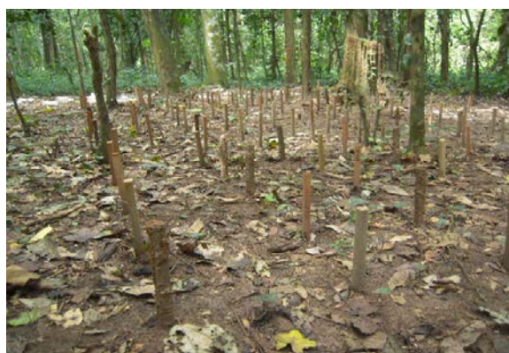
Figure 7.4: Test samples infested with termite
