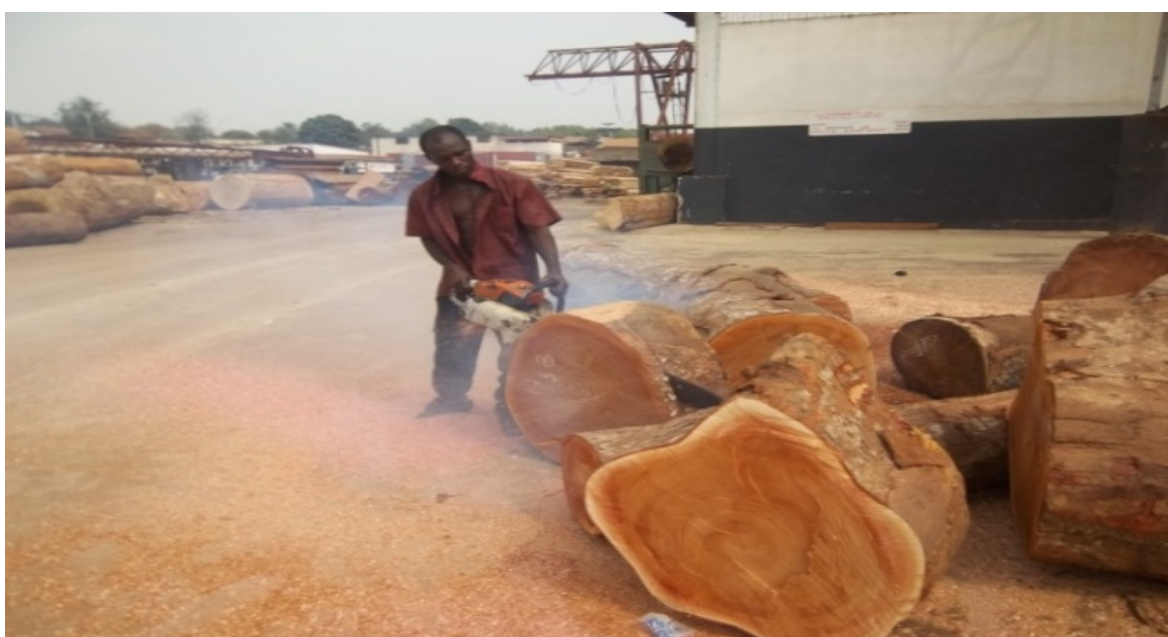
Figure 4.5: Cross cutting of logs and removal of disc for at LLL logyard
