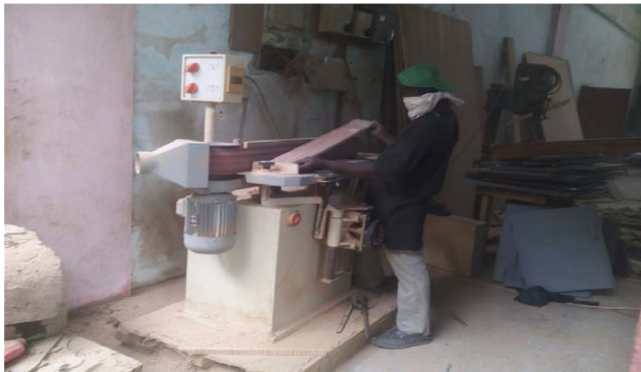
Figure 3.2: Materials being sanded at FORIG Workshop
