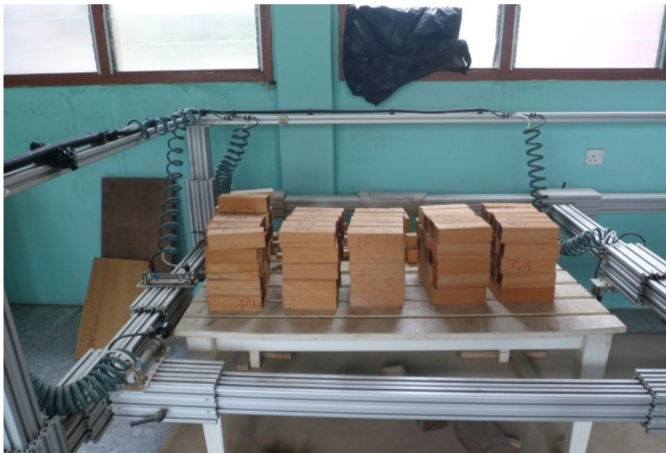
Figure 6.2: sample of mahogany for mechanical properties test
