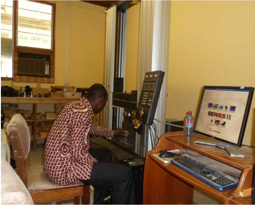
Figure 6.1: Testing of clear samples using Instron testing machine
