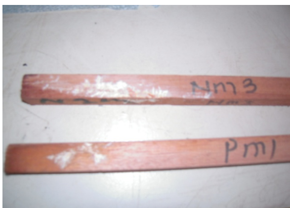
Figure 7.5: Test samples infected with fungi from the graveyard test
