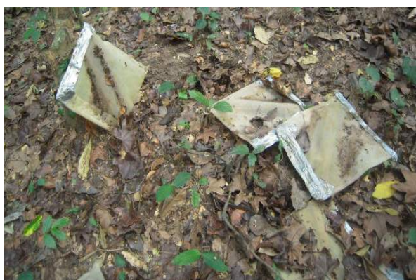
Figure 7.3: Termite exclusion test samples on the forest floor
