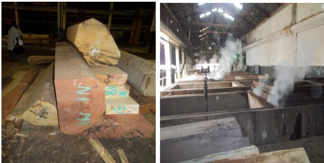
Figure 4.9: Preparation of flitches and heating of logs or veneer production
