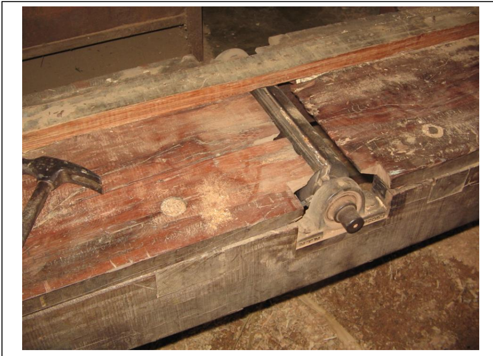
Fig. 4 Equipment in most micro and small firms are usually locally fabricated and have no safety features
