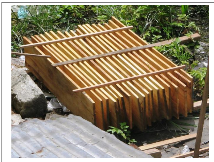
Fig. 3a and 3b Modes of drying of raw materials used by micro and small firms – air drying and with the use of improvised dryer
