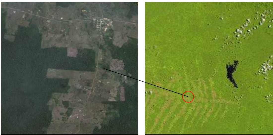
Figure 3. Detection of forest clearing using IKONOS (4 m) and Landsat 5 (30 m) satellite data
