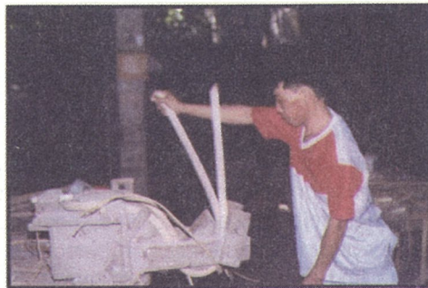
Figures 31 and 32. Bending of rattan poles using a jig.
