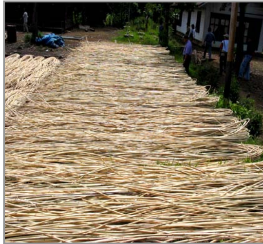
Figure 3.7. Drying rattan canes in the sun for 3-4 days to have water content 10-12%
