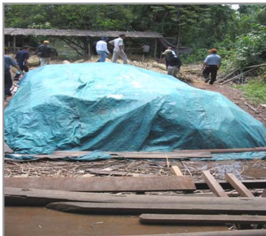
Figure 3.6. Fumigation of rattan canes using sulfur smoke for 24 hours
