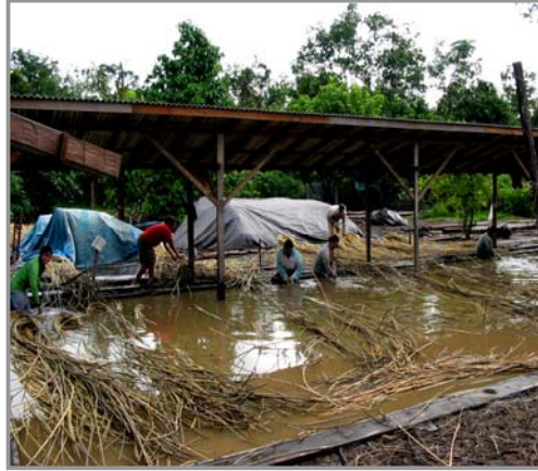
Figure 3.4. Wash after deglazing and then dry before fumigate for small diameter cane.
