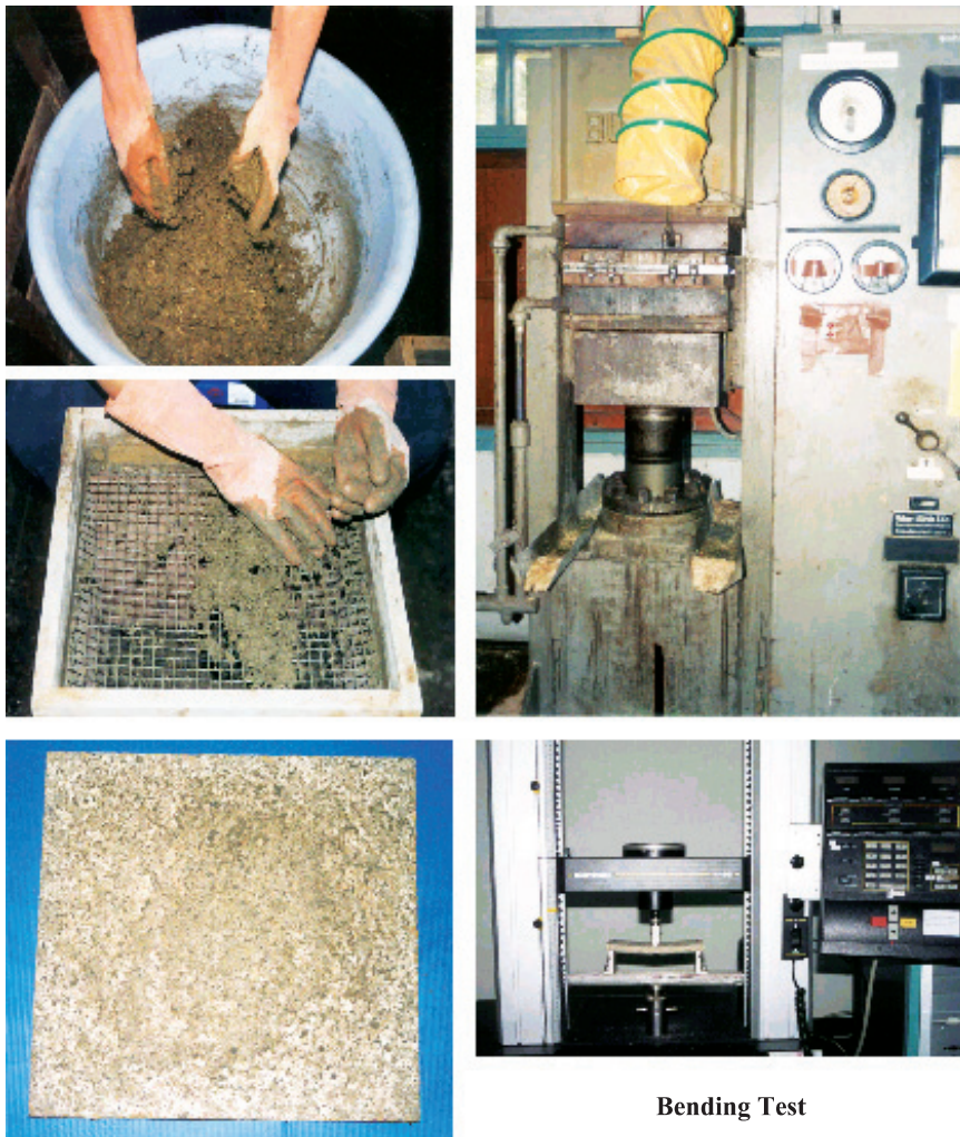
Figure 1. Preparation and testing of bamboo cement board.
