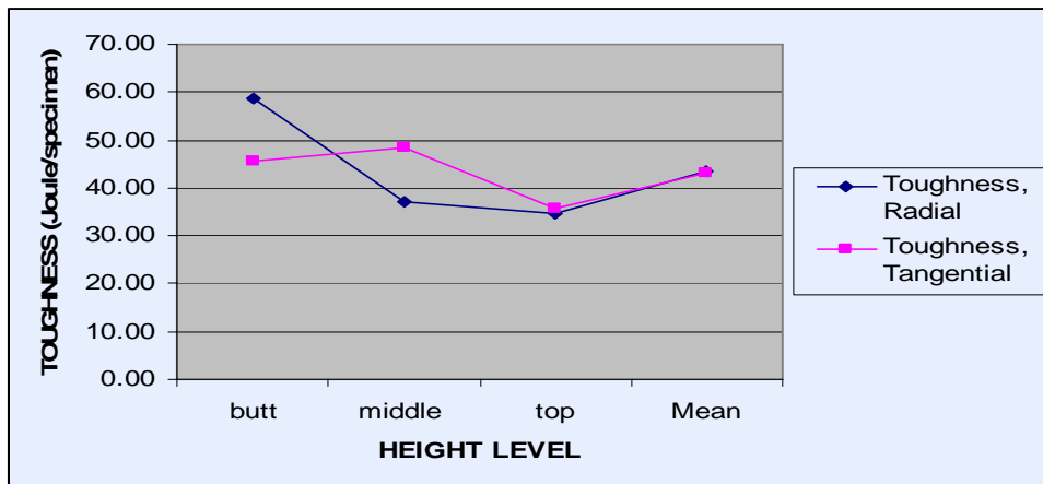
Fig. 25. Toughness of A. macrophylla at different height levels.
