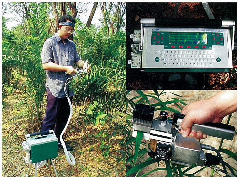
Figure 3. LI-6400 portable photosynthesis system (LICOR Inc.) for leaf photosynthesis measurements of Calamus viminalis in the field.
