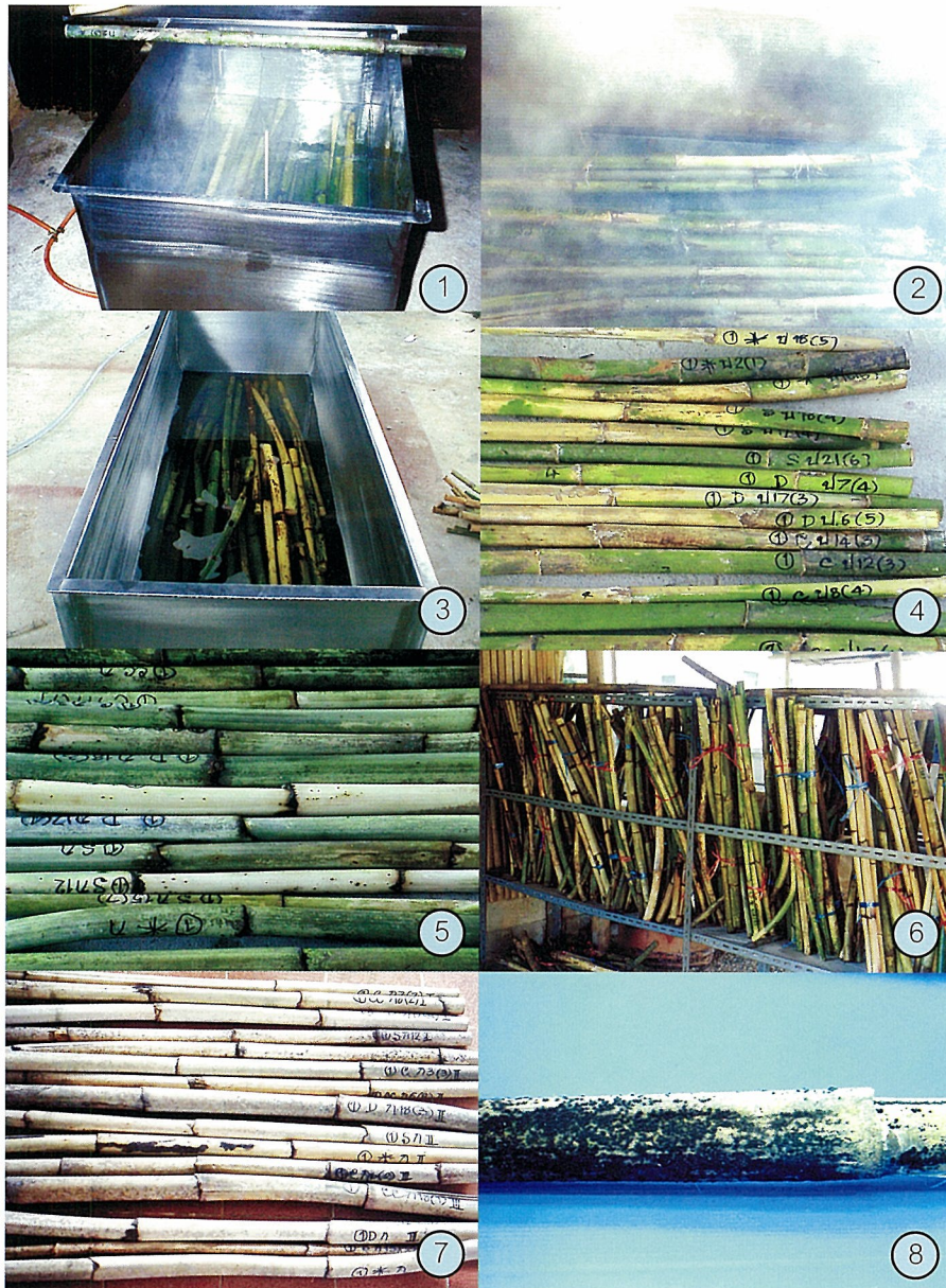
Annex Figure 2. Treatment to rattan material in the present study, (1) – (2) oil curing treatment, (3) immersion in Boron compounds, (4) rattan canes before treatment, (5) rattan canes after oil curing, (6) treated rattan canes are air-dried vertically on the rack, (7) rattan canes after air drying, and (8) rattan cane is infested by staining fungi.
