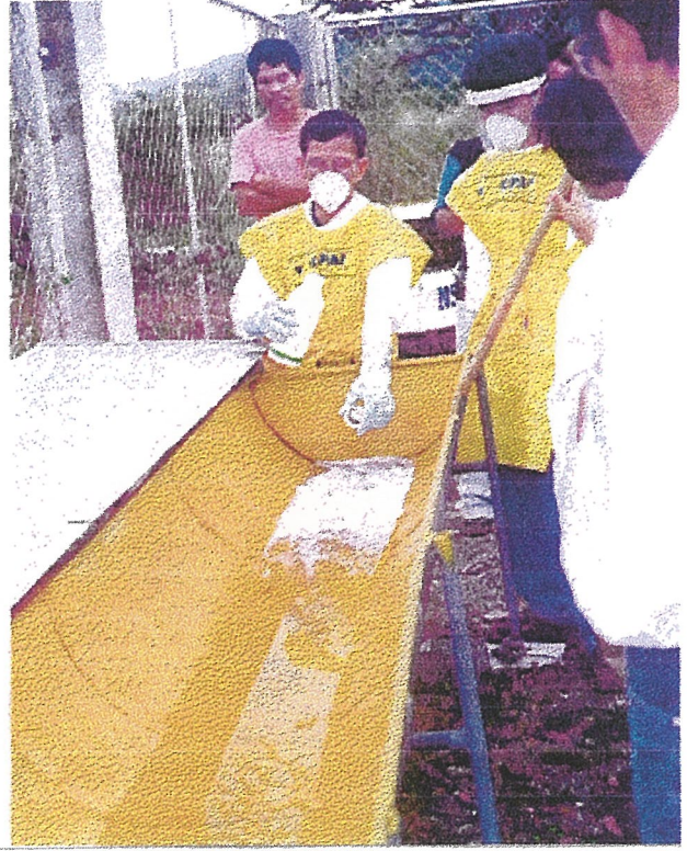
Preparation of chemicals in a dipping vat made of steel drum split into halves and welded along the length.
