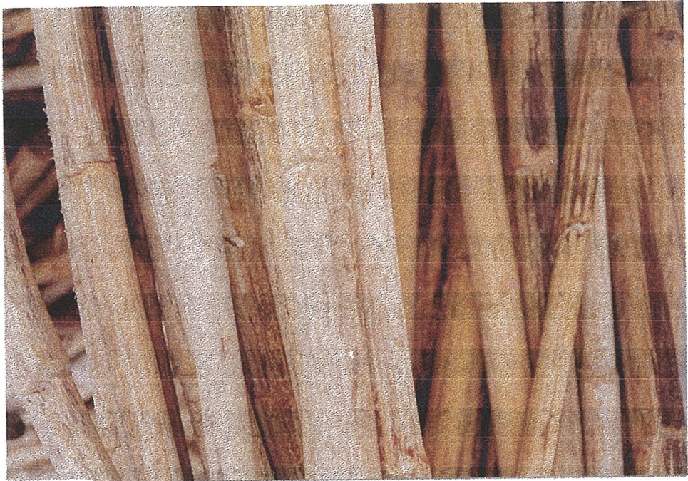
Untreated scraped rattan with black stains.
