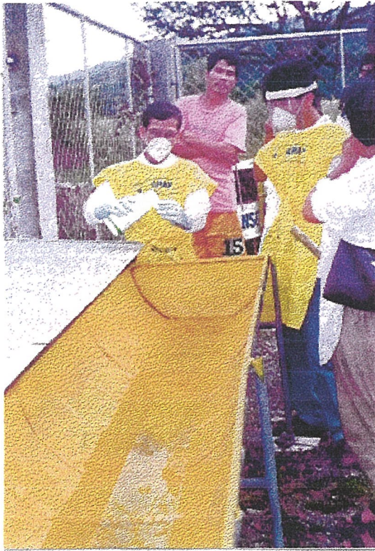
Preparation of chemicals in a dipping vat made of steel drum split into halves and welded along the length.
