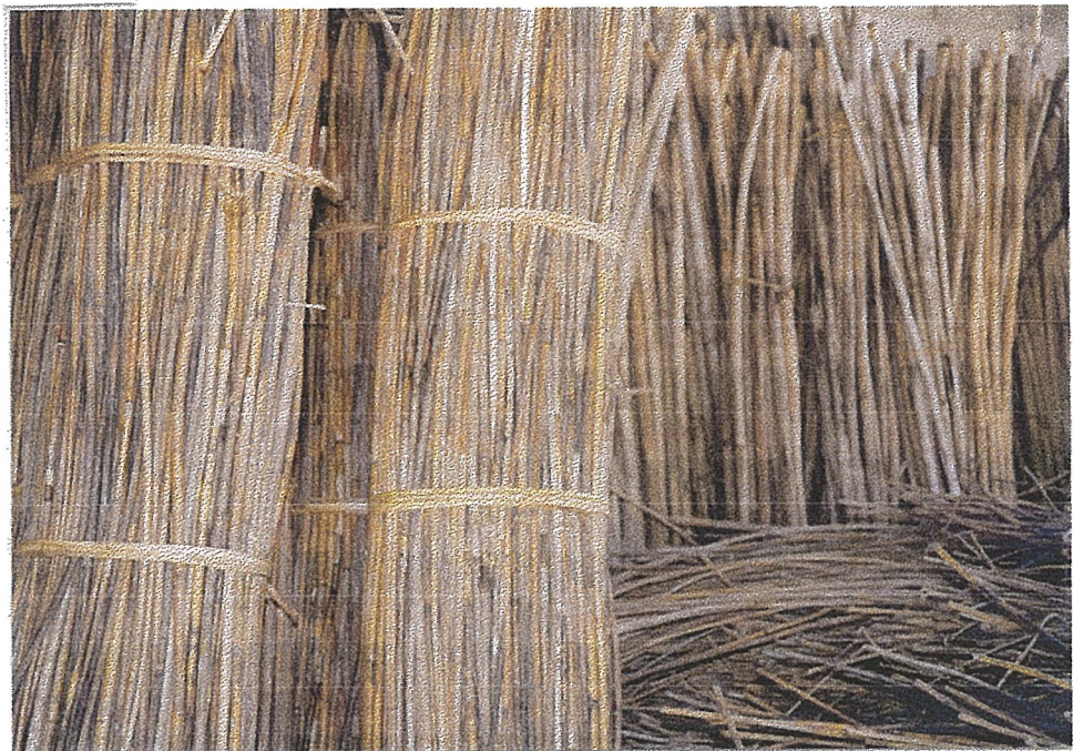
Untreated unscraped rattan poles with black stain.
