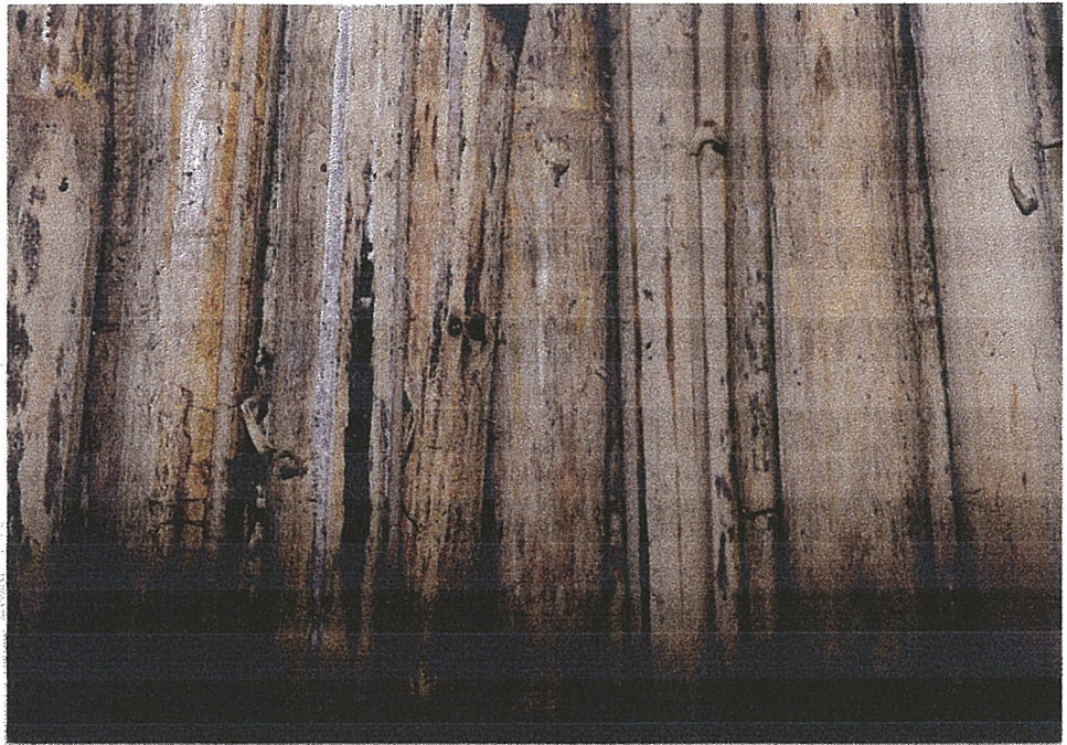
Stored Rattan poles with dark colored fungal stain.
