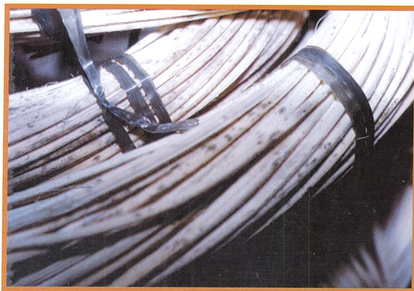
Rattan canes with molds and staining fungi. Proper storage was recommended.
