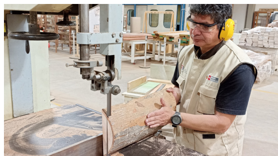
Preparing specimens for wood testing in the CITEMADERA laboratory. © CITEMADERA
