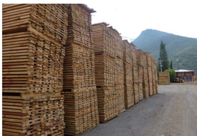
Open air drying of wood, Mexico. Photo: Industria Forestal Pueblos Mancomunados
