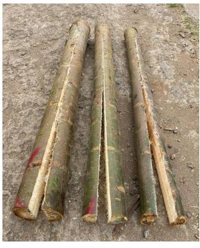
Eighteen-month-old balsa logs subjected to a cracking test, Northern Region of Costa Rica. © Róger Moya
