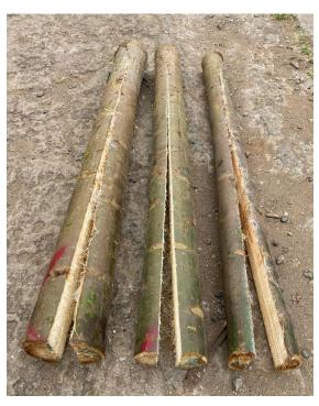
Eighteen-month-old balsa logs subjected to a cracking test, Northern Region of Costa Rica. © Róger Moya
