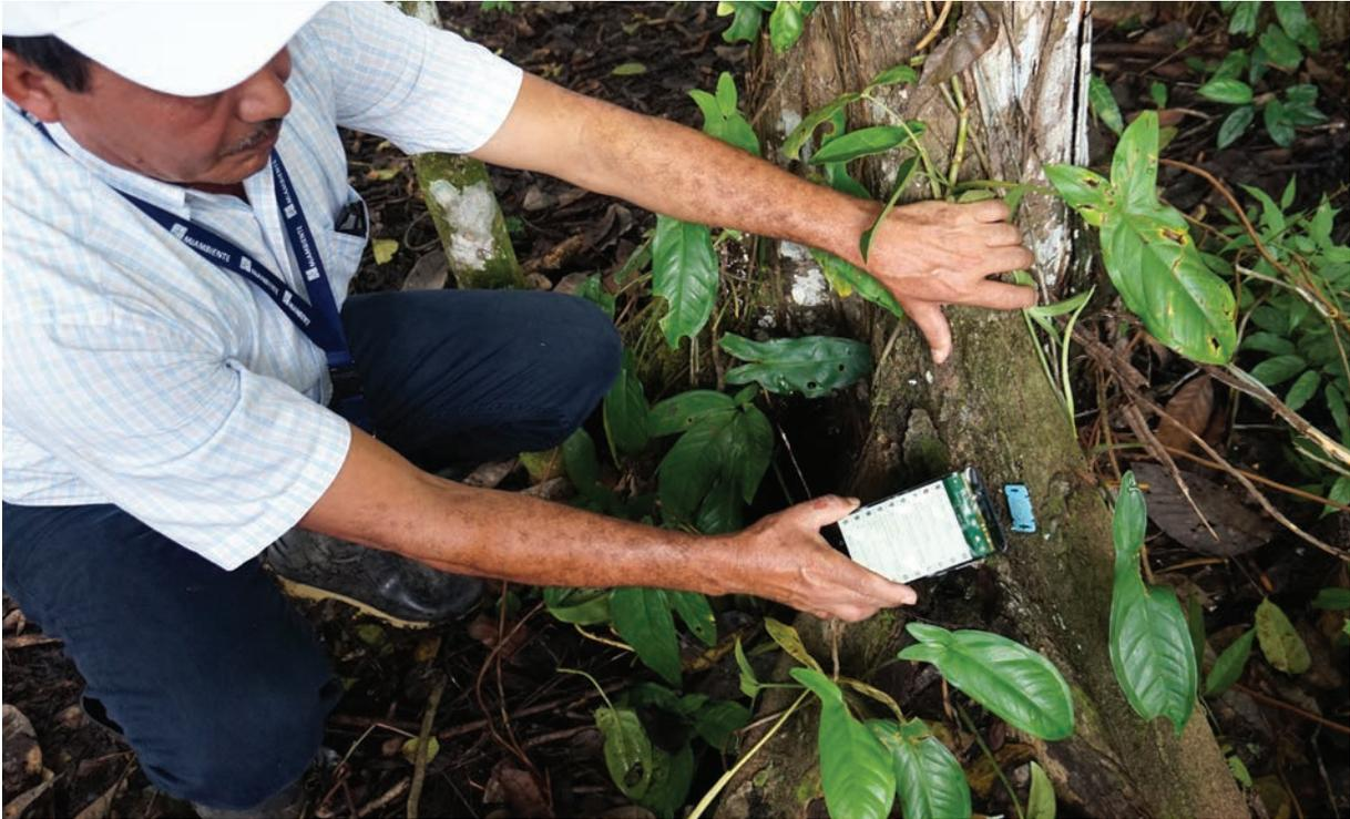
*A field-officer scans a tag attached to a tree in a forest in Darién, Panama. Panama's new timber traceability system, developed as part of an ITTO project, enables the tracking of timber from the forest to the mill and beyond. Photo: R. Carrillo/ITTO*
