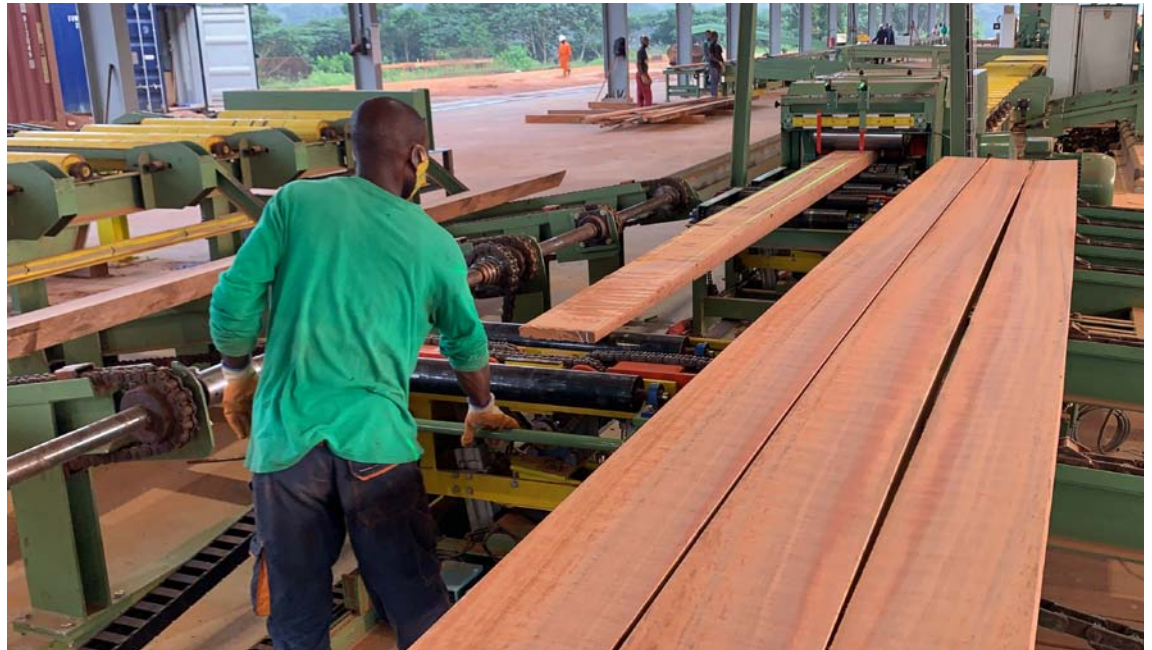
Precious wood: These azobe boards have been sawn in a new Precious Woods plant in Gabon. Photo : © Precious Woods
