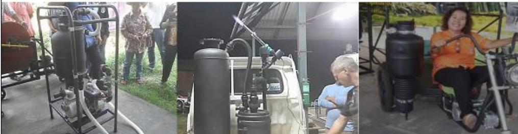
Using of bamboo charcoal as a raw material to produce syngas to be used for renewable energy instead of oil in water pump, motorcycle, pickup car and electrical generator.
