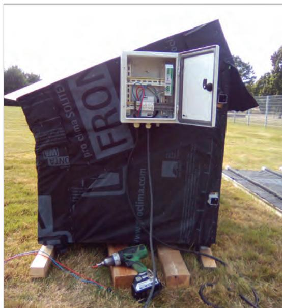
**Dry run:** A prototype solar collector being built at the Laboratory of Studies and Research on Wood Materials in Epinal, France, to test its role in wood-drying. *Photo: Merlin Simo-Tagne*
