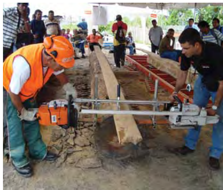
Instructors demonstrate the use of guides in chainsaw milling to increase wood recovery as part of training conducted under ITTO project PD 687/13 Rev.1 (I). Photo: P. Bholanath/Guyana Forestry Commission
