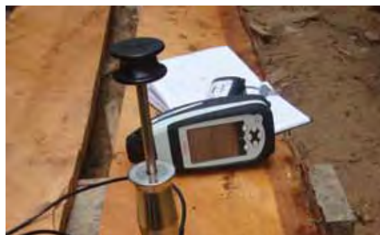
This equipment uses near infrared spectroscopy to identify wood as part of efforts to monitor the mahogany trade in Brazil. Photo: Laboratório de Produtos Florestais
