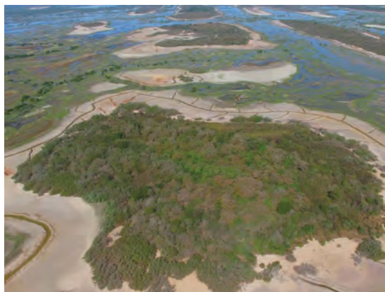
Plain drains: Canals have been installed in this degraded mangrove area to improve water flows, thereby assisting the restoration process. Photo: Ernesto Beltrán García
