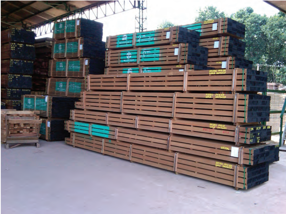
Gun barrel straight: Certified dressed bullet wood ( Manilkara bidentata ) sawnwood, graded for export. Photo: www.ecosdelbosque.com
