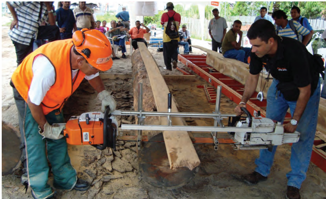
Guide on guiding: Instructors demonstrate the use of guides in chainsaw milling to increase wood recovery. Photo: P. Bholanath/GFC
