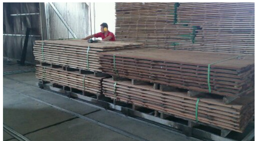
Flat to the floor: Lumber of lesser-used species prepared for conventional kiln-drying produced in an industrial pilot operation. Photo: I. Jankowsky
