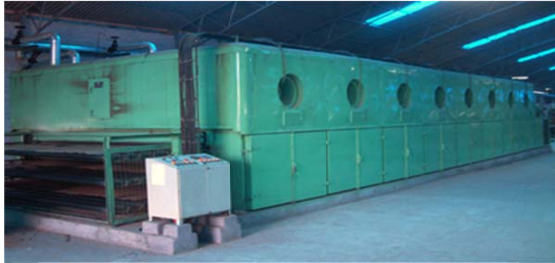
Figure 8. Continuous veneer drying.
