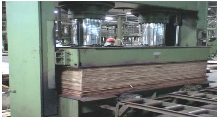
Figure 11. Cold pressing process.
