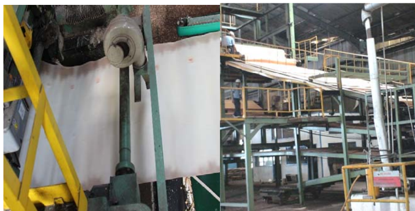
Figure 7. Reeling and unreeling of veneer
