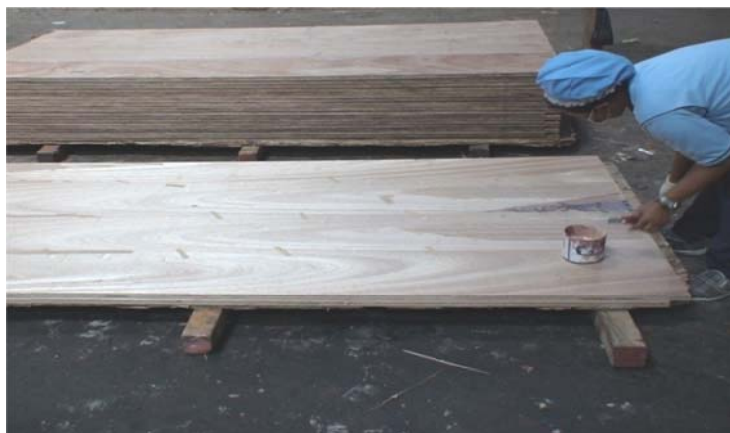
Figure 13. Plywood putty process.
