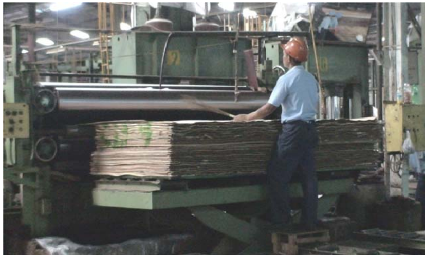
Figure 10. Glue spreading process.
