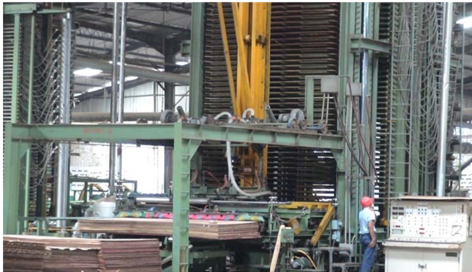
Figure 12. Hot pressing process.
