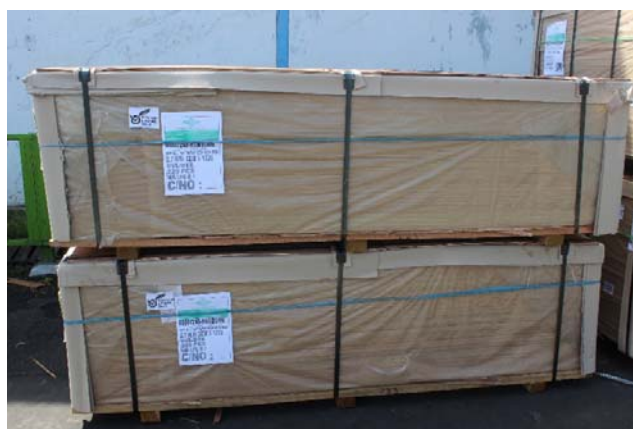
Figure 14. Packing of plywood for storage/shipment
