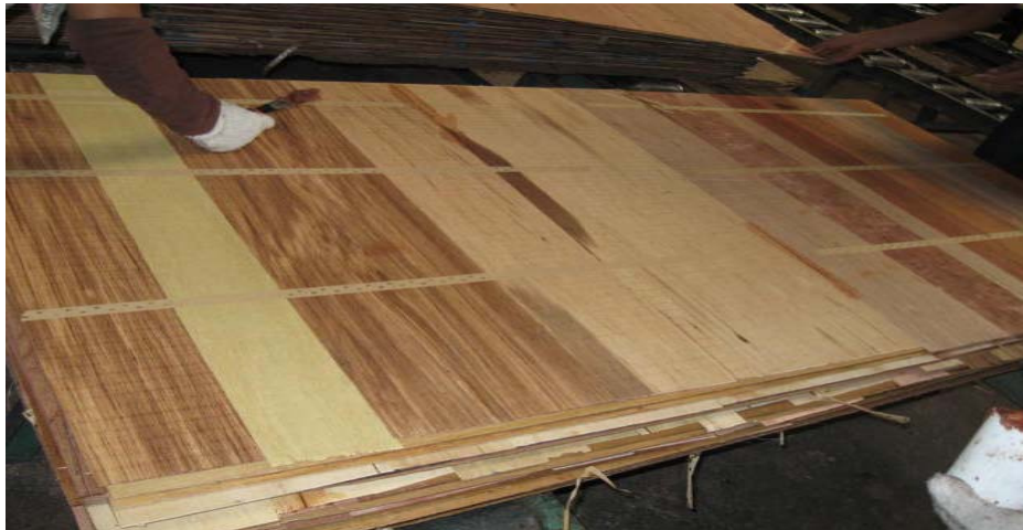
Figure 9. Veneer selection and repairing
