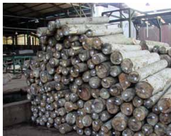
Small is beautiful: Plantation-grown small-diameter logs used for core-layer veneer for plywood in a mill in West Java, Indonesia. Photo: Zhou, Y.
