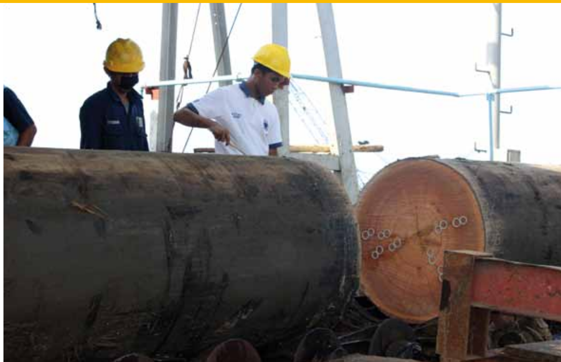
Cradle: Plastic figure-8 nails are applied to meranti plywood logs to reduce end-splitting in a log yard in Probolinggo, Indonesia. Photo: MY Massijaya
