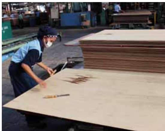
Flaw repair: A worker repairs a meranti plywood veneer sheet on the factory floor. Photo: MY Massijaya
