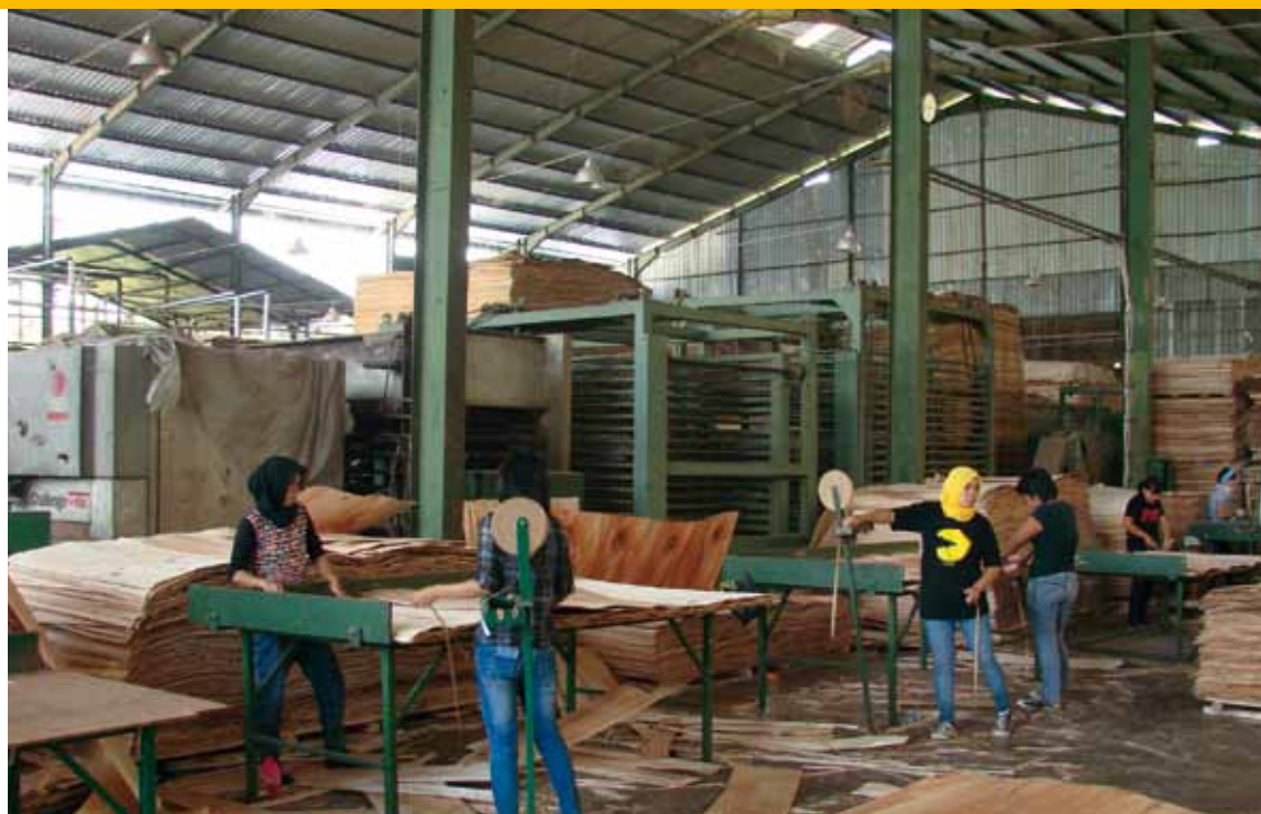
Labour-intensive: Repairing and joining veneer made from small-diameter logs in a mill in West Java, Indonesia. Photo: Zhou, Y.
