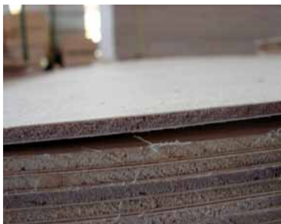
Core value: SDL veneer is the major (central) part of the plywood.
