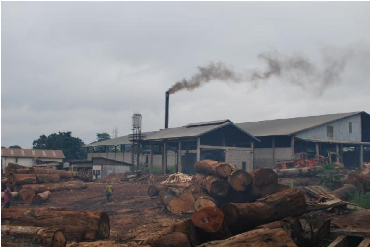
Fig. 9: Furnace; burning wood to produce steam for heating kiln dryers
