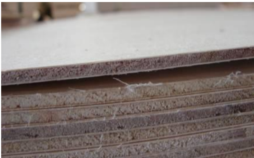
The SDL veneer is the major proportion of the plywood (Central part)
