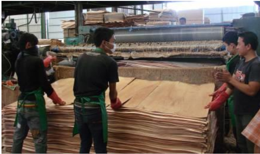
Labor intensive works in plywood layup section
