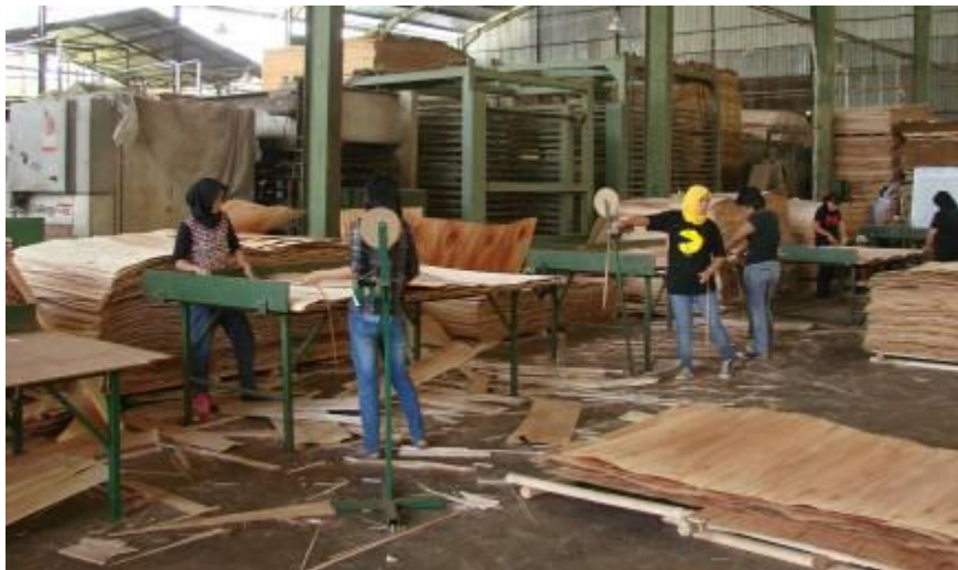
Repairing and jointing of veneer from SDL plantation resources
