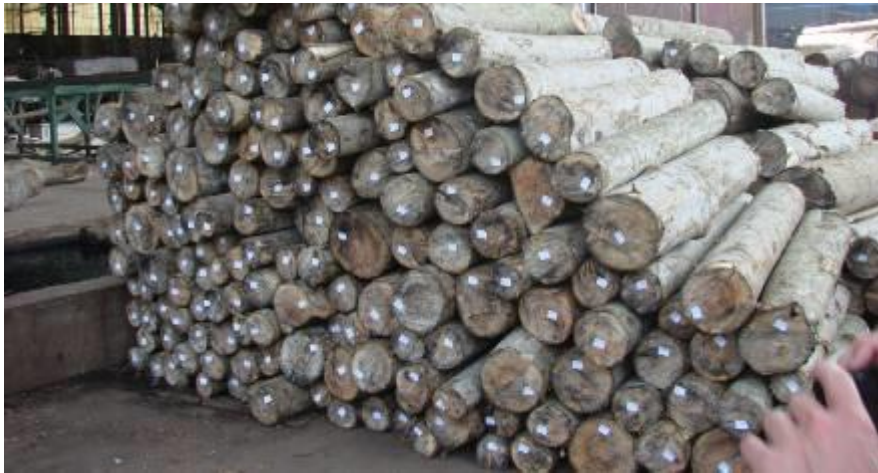
The plantation SDL for core layer veneer of plywood
