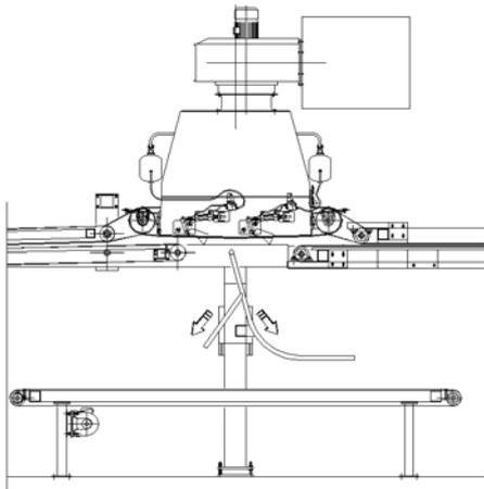
part of the log, peeled thickly, directly to the clipper. The rotary type clipper, with scanner and electronic control, cuts off veneer defects automatically and optimizes veneer clipping. The clipper speed is synchronized with the peeling speed and the veneer is therefore worked in real time.
