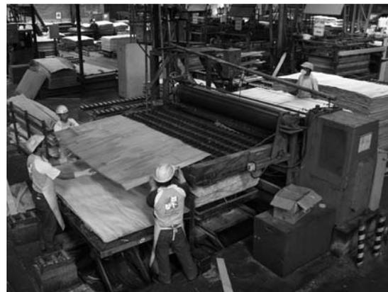
Two automatic trimming lines, one per mill, square each board to perfection (see Figure 80).
