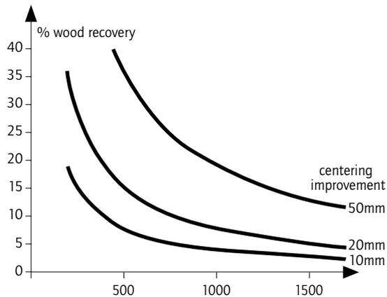
For this reason, this company is suggesting the installation of XY electronic centering devices to ensure extraction of the maximum value of tropical logs, as has been common practice when processing small-diameter plantation logs.
