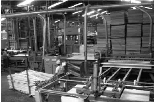
At the end of the production process (Figure 81), there are three sanding lines with two heads at the bottom and three heads in the top; these produce a final product with a very smooth surface.
