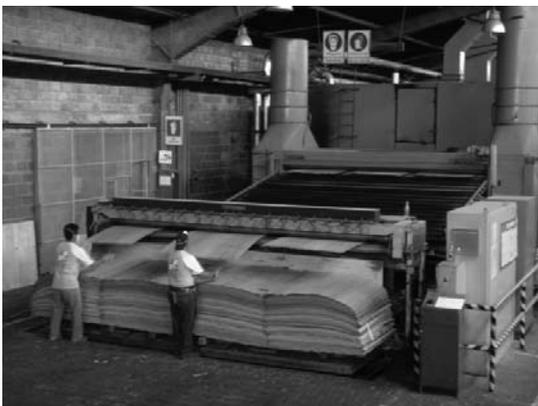
Six veneer dryers of different brands are in operation, three shifts per day, six days per week. Some are equipped with moisture meters at the dry end to avoid over-drying. A series of five core composers per mill are used to maximize recovery and quality.
