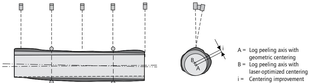
One of the most important current issues is to maximize log utilization in order to obtain the highest recovery. In this regard, some machinery manufacturers have paid attention to finishing with log cores at the end of the peeling process with the smallest possible diameter through the use of different devices mounted
