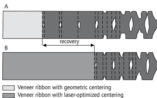
As an example, peeling a log core of 100 mm diameter down to 40 mm diameter, peeled at 2 mm thickness, you recover 3.3 m of core-quality veneer. On the other hand, if working with a block of 1,000 mm diameter using an XY electronic centering device, centering accuracy can be improved by 20 mm compared to standard centering, allowing the recovery of some 15.5 m of good-quality veneer if peeled at 2 mm thickness (see figures 63a-b).
