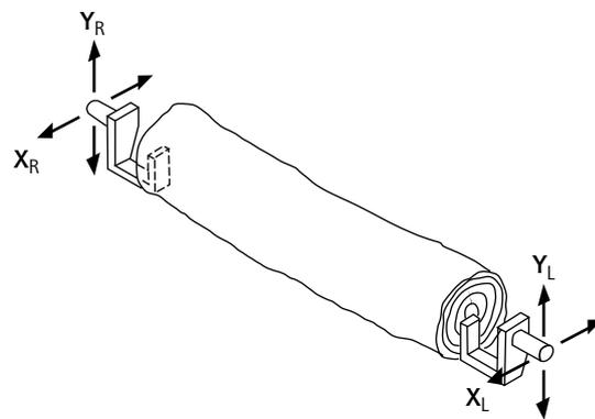
In this way the block is identified and measured at different sections according to length. The information coming from the lasers is sent to a computer, which processes the coordinates and, through an iterative calculation system, determines the new block axis. Consequently the X and Y positions are calculated and set on the log ends, right and left (see Figure 66).
