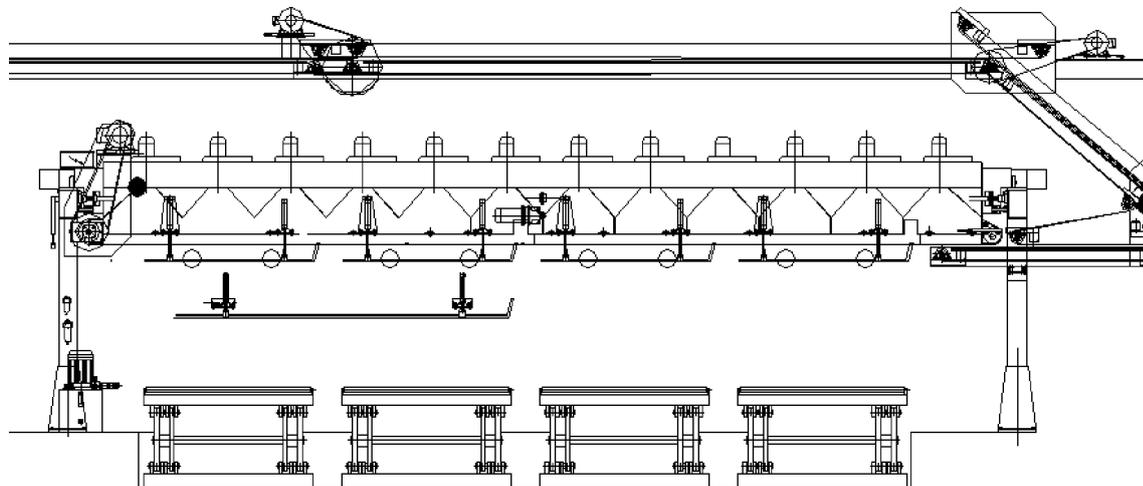
Figure 70. Twin Rotax® Clipper Twin-Knife System
