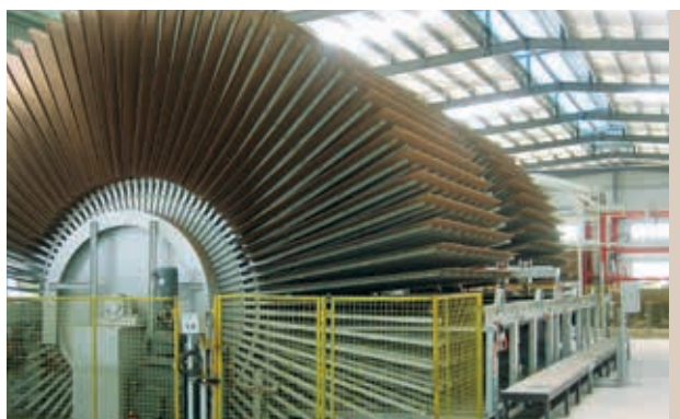
A fiberboard cooling system at the Hongtai wood-processing company, China. Photo: J. Claudon, ITTO
