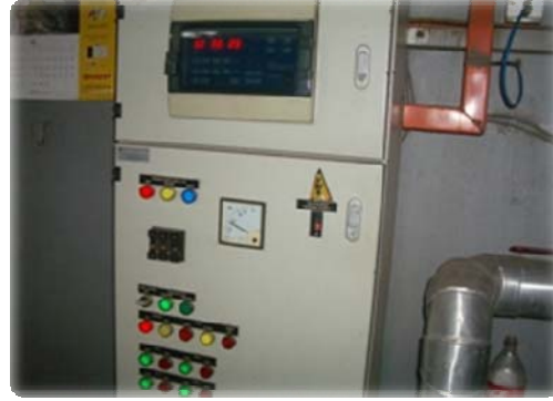
Computerized control of kiln-drying schedule by Worldtrend
