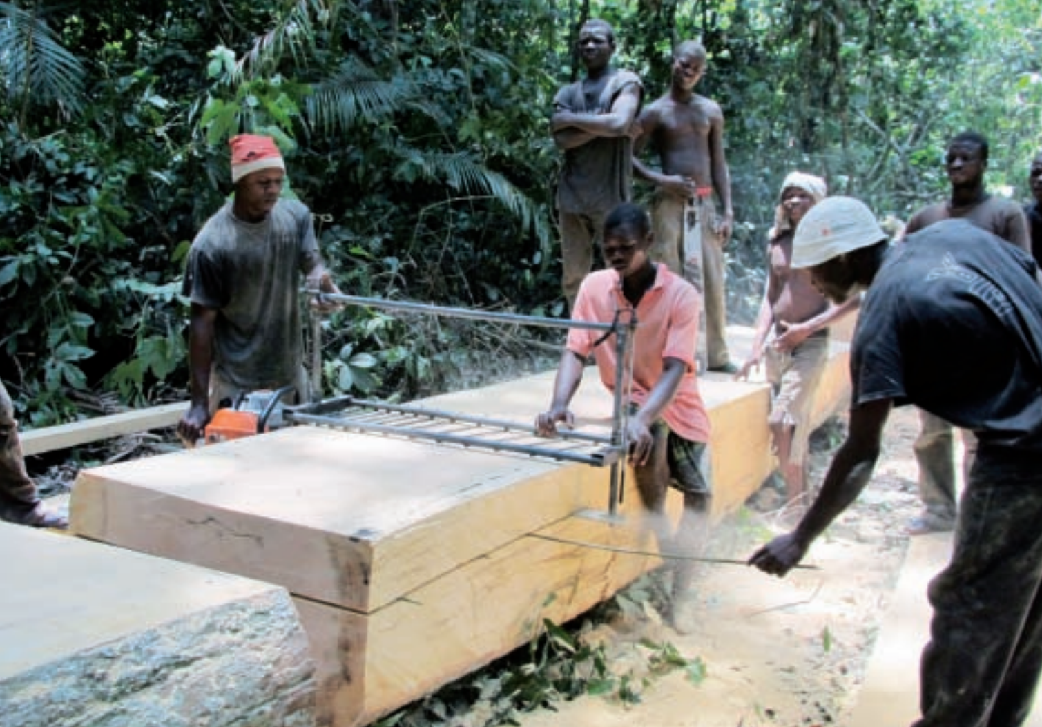
Portable chain-sawmill, Central African Republic. © FAO/M. Vandenhoute
