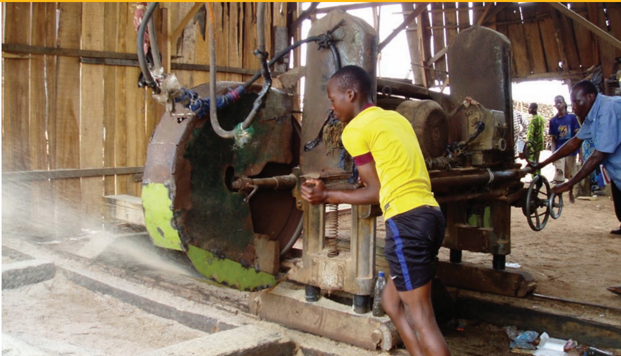
Manpower: Operators push a horizontal bandsaw through a log. Photo: V. Molinos
