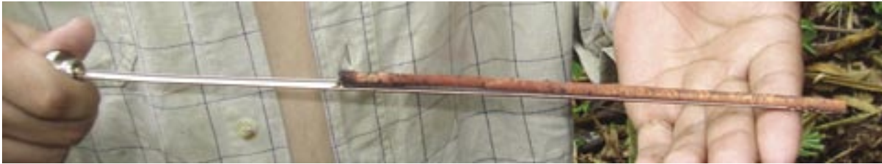
Heart rot: A timber sample of a standing mahogany tree obtained with the Pressler borer. Photo: I. Lombardi
