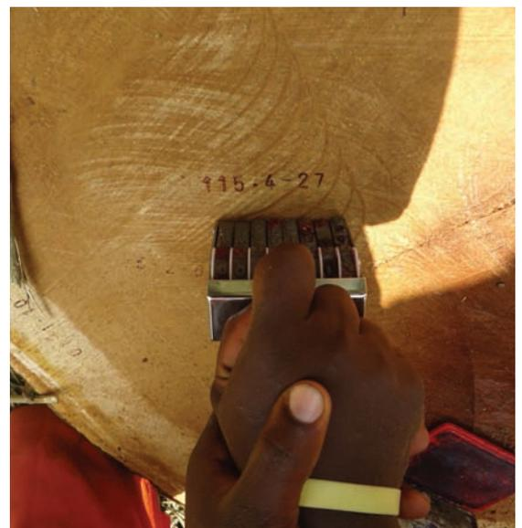
**...and numbered:** Device for numbering sawn timber. Photos: K.S. Bobo
