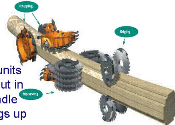
Other multi-station units such as R250 duo cut in two planes, can handle sweep in logs for logs up to 350 mm diameter
