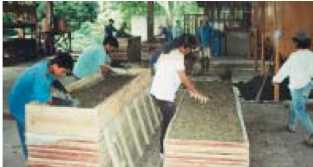
**Small-scale wood-wool cement board plant in the Philippines showing the process of forming boards by hand**
