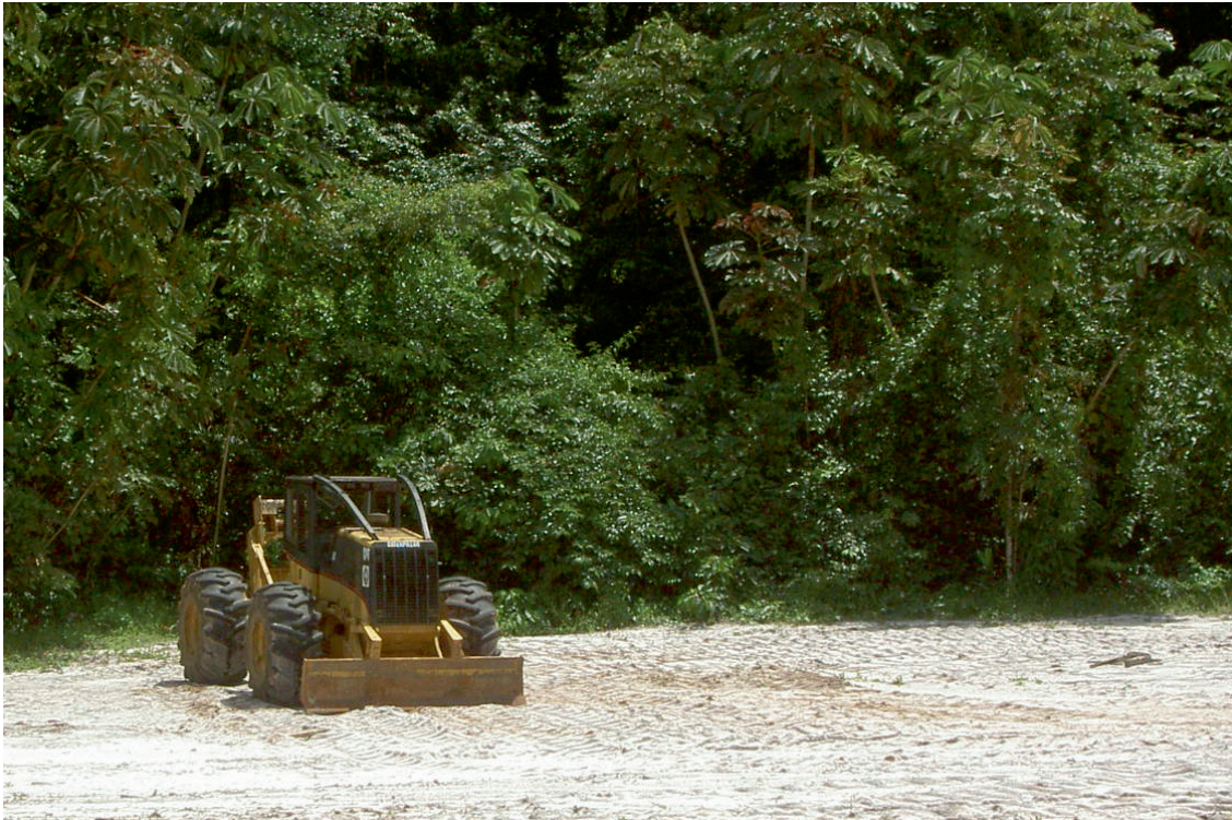
Low impact: Wide-tired tractor used in FTCI's RIL training. Photo: E. López Rojas
