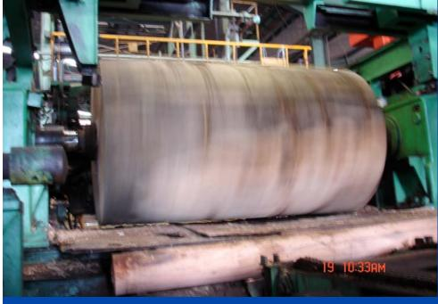
Traditional peeling, the core diameter left Φ=140-160mm
